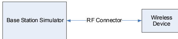
Figure 8-1 Power Measurement Setup
