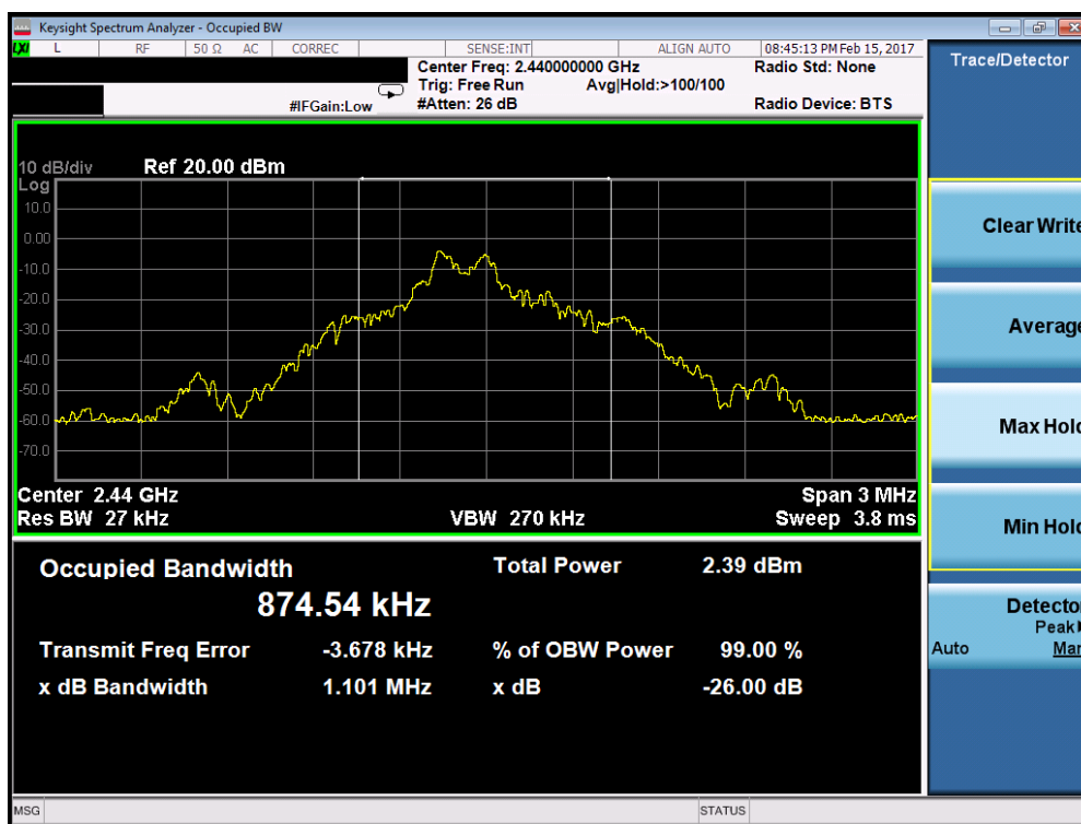
Plot 7-1. Occupied Bandwidth Plot (ANT+ – Ch. 39)
