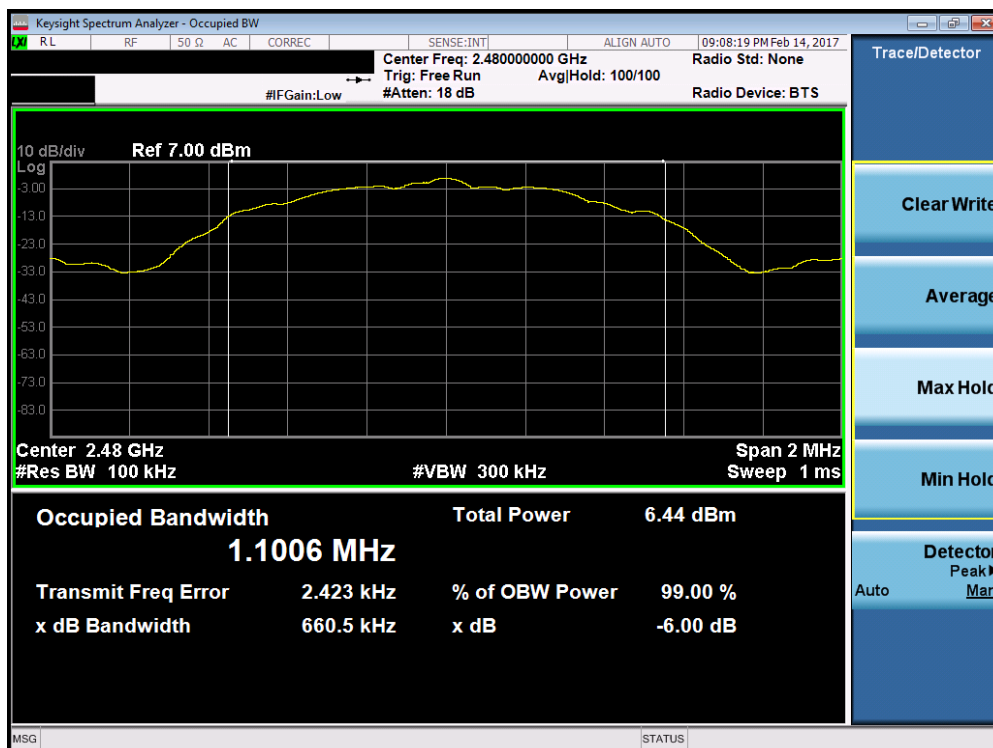
Plot 7-3. 6dB Bandwidth Plot (Bluetooth (LE) – Ch. 39)
