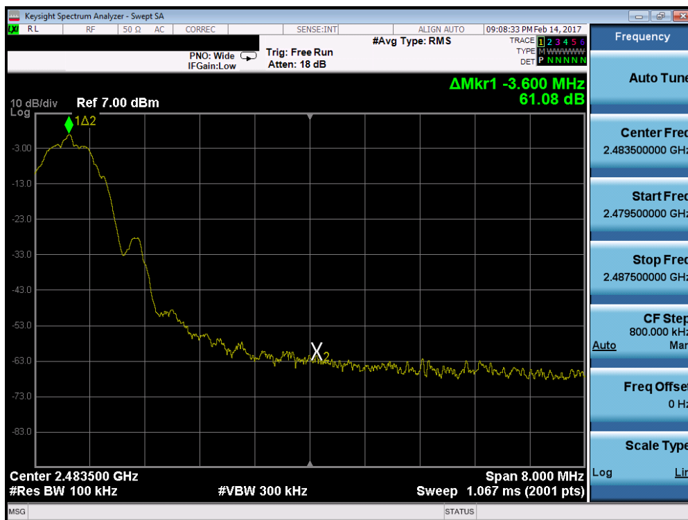
Plot 7-11. Band Edge Plot (Bluetooth (LE) – Ch. 39)
