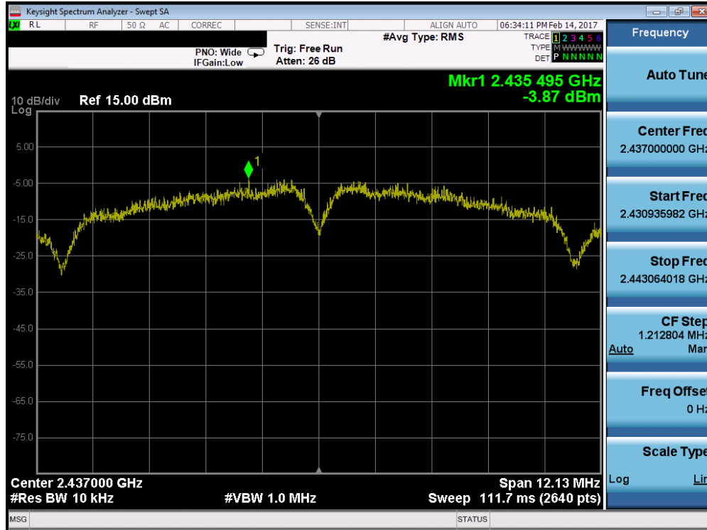
Plot 7-29. Power Spectral Density Plot (802.11b – Ch. 6)
