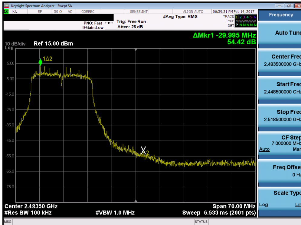
Plot 7-48. Band Edge Plot (802.11n (2.4GHz) – Ch. 11)
