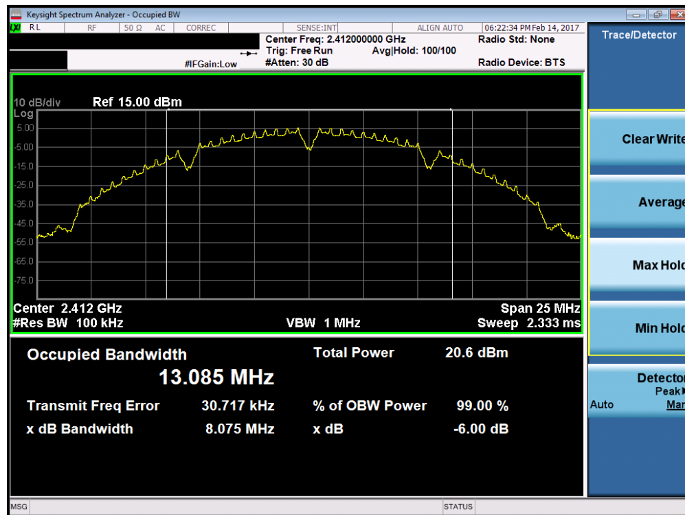
Plot 7-1. 6dB Bandwidth Plot (802.11b – Ch. 1)
