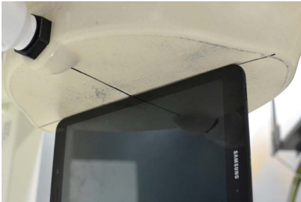
SAR Test Setup Photo 8: Left Edge at 0.0 cm
