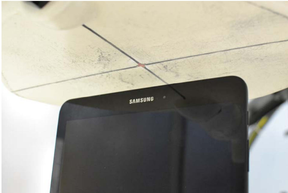
SAR Test Setup Photo 4: Top Edge at 1.9 cm
