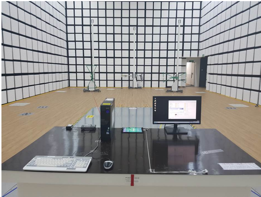
[ Radiated Disturbance for Below 1 GHz – Front ]
