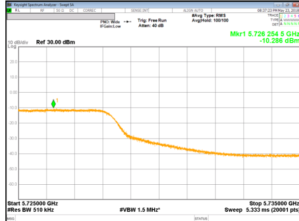
11n HT40 Mode UNII 3 PSD Antenna 1
