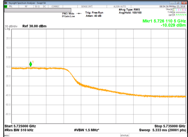
11n HT40 Mode UNII 3 PSD Antenna 2
