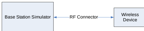
Figure 8-1 Power Measurement Setup
