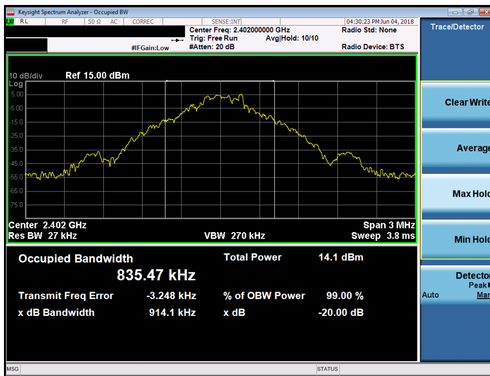
Plot 7-1. 20dB Bandwidth Plot (Bluetooth, 1Mbps – Ch. 0)
