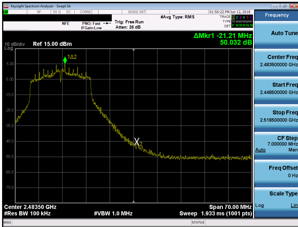
Plot 7-48. Band Edge Plot SISO ANT2 (802.11n (2.4GHz) – Ch. 11)
