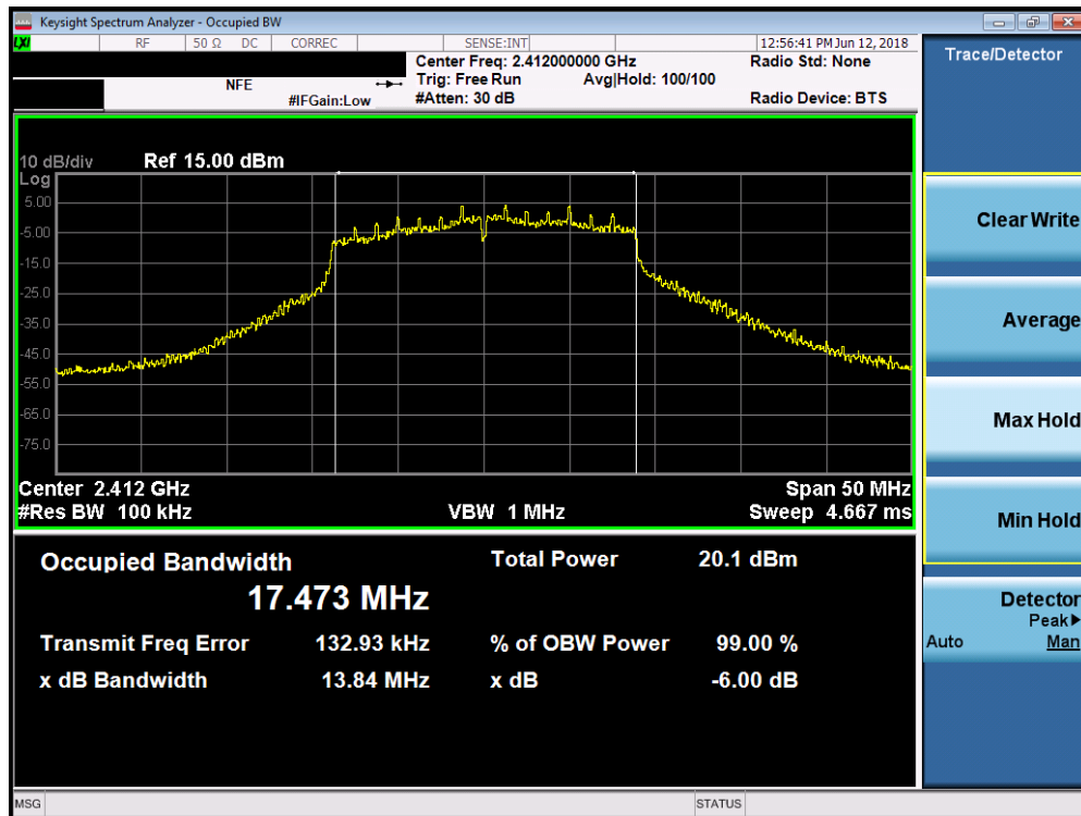
Plot 7-7. 6dB Bandwidth Plot SISO ANT1 (802.11n (2.4GHz) – Ch. 1)
