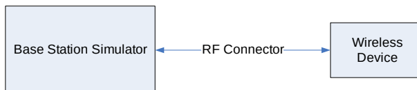
Figure 8-1 Power Measurement Setup
