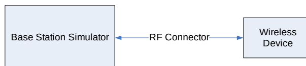
Figure 8-1 Power Measurement Setup
