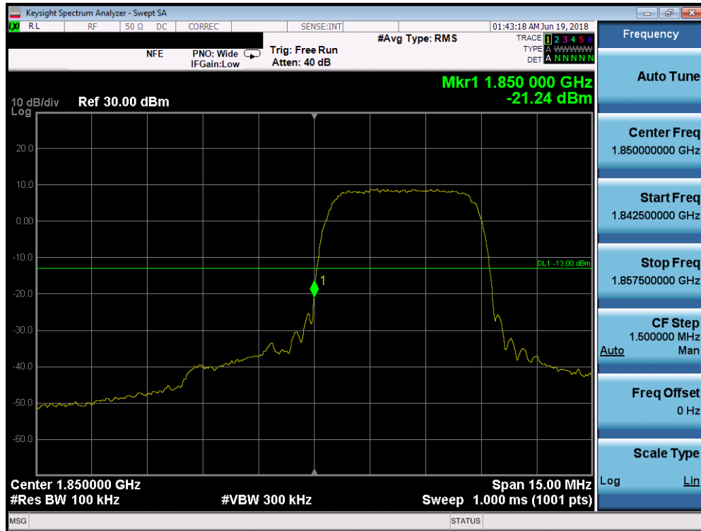
Plot 7-43. Band Edge Plot (PCS WCDMA Mode - Low Channel)
