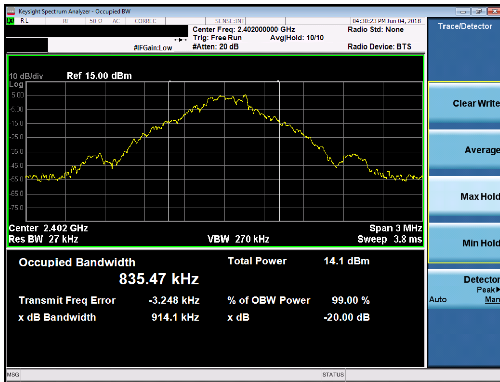
Plot 7-1. 20dB Bandwidth Plot (Bluetooth, 1Mbps – Ch. 0)
