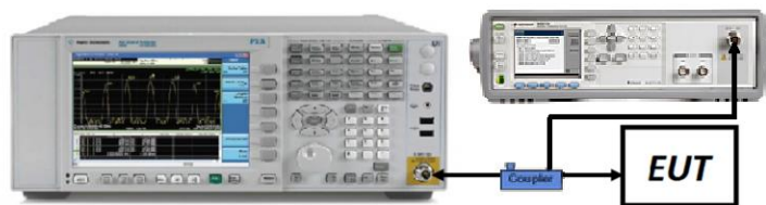
Figure 7-5. Test Instrument & Measurement Setup
