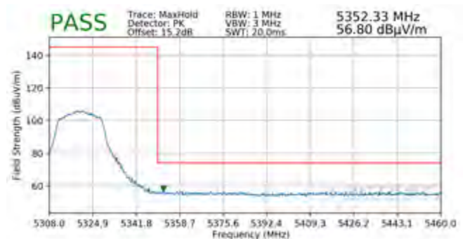
Plot 7-217. Radiated Upper Band Edge Plot (Peak – UNII Band 2A)
