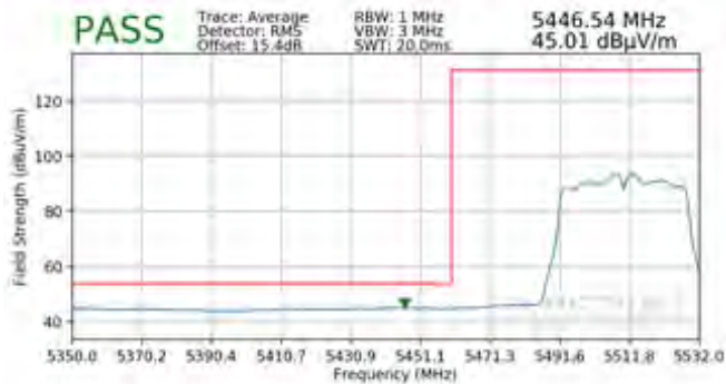
Plot 7-204. Radiated Lower Band Edge Plot (Average – UNII Band 2C)
