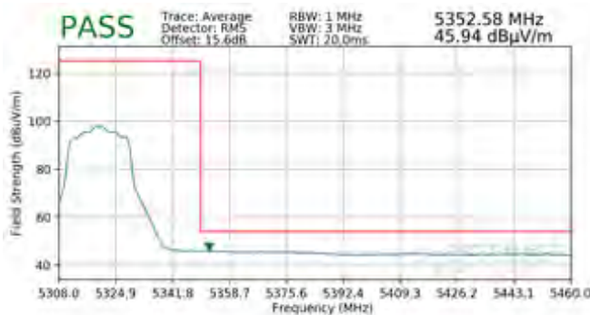
Plot 7-174. Radiated Upper Band Edge Plot (Average – UNII Band 2A)
