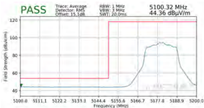
Plot 7-193. Radiated Lower Band Edge Plot (Average – UNII Band 1)
