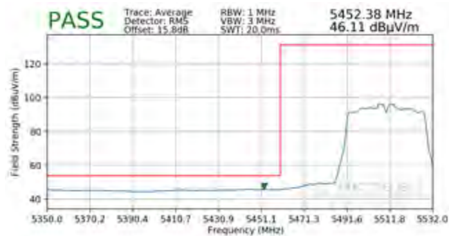
Plot 7-232. Radiated Lower Band Edge Plot (Average – UNII Band 2C)
