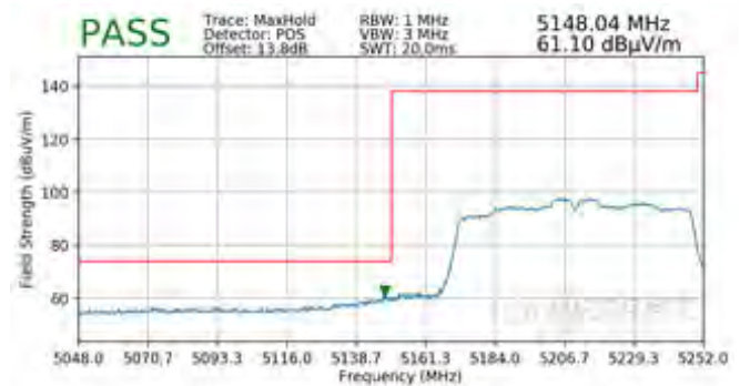
Plot 7-236. Radiated Lower Band Edge Plot (Peak – UNII Band 1)
