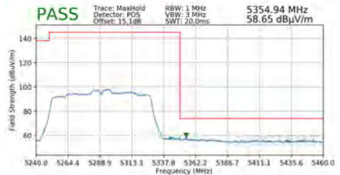
Plot 7-210. Radiated Upper Band Edge Plot (Peak – UNII Band 2A)
