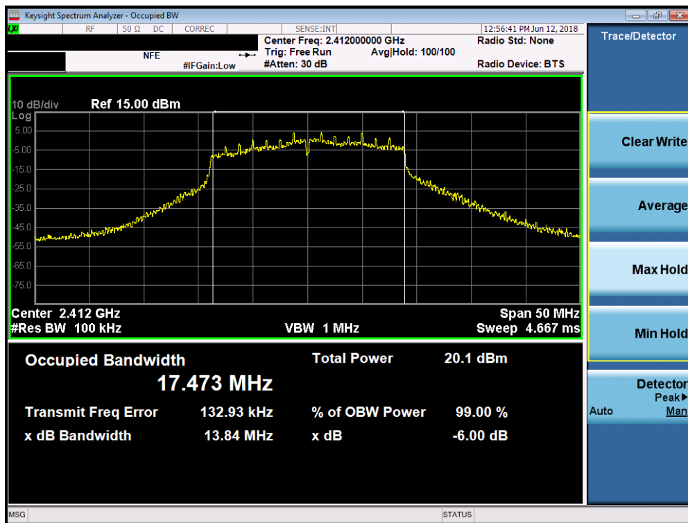
Plot 7-16. 6dB Bandwidth Plot SISO ANT1 (802.11n (2.4GHz) – Ch. 1)
