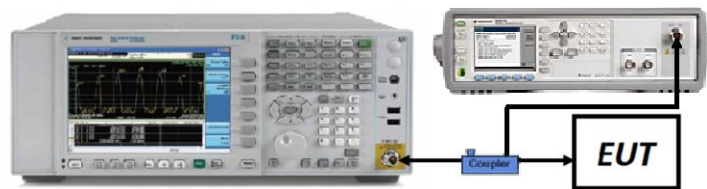
Figure 7-3. Test Instrument & Measurement Setup
