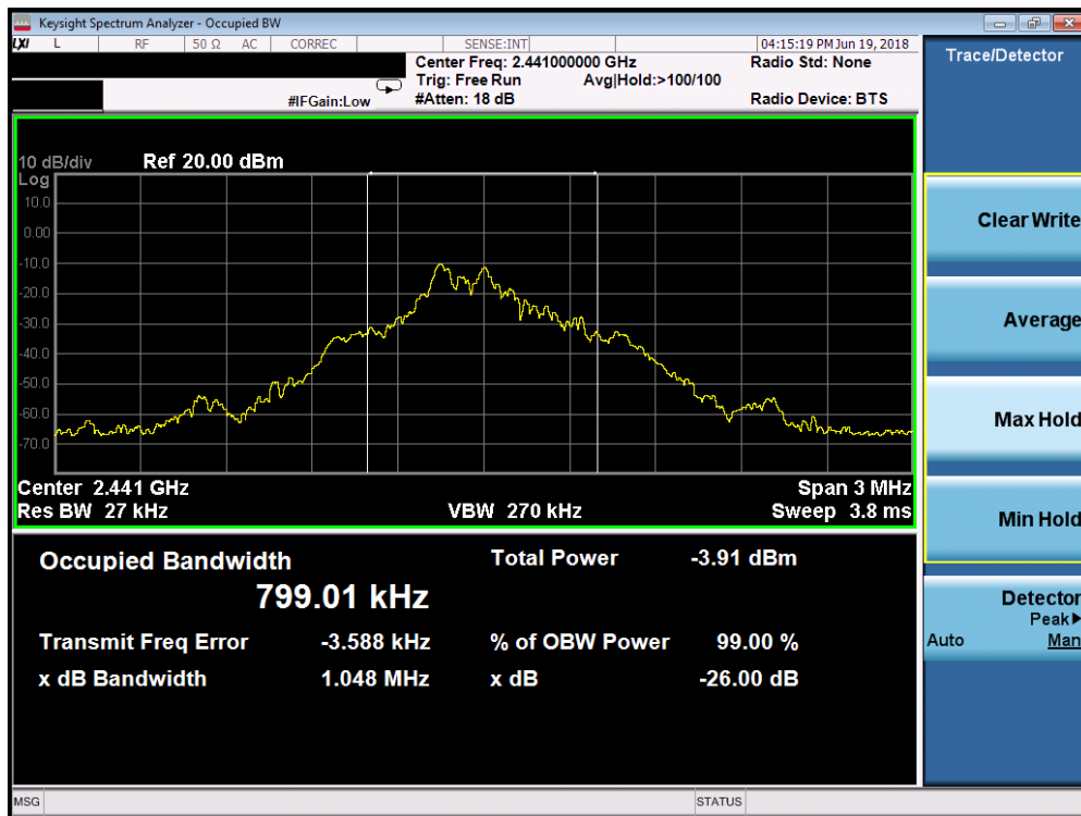
Plot 7-1. Occupied Bandwidth Plot (ANT+ – Ch. 39)
