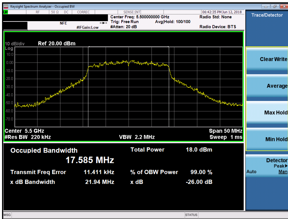
Plot 7-22. 26dB Bandwidth Plot (20MHz BW 802.11n (UNII Band 2C) – Ch. 100)
