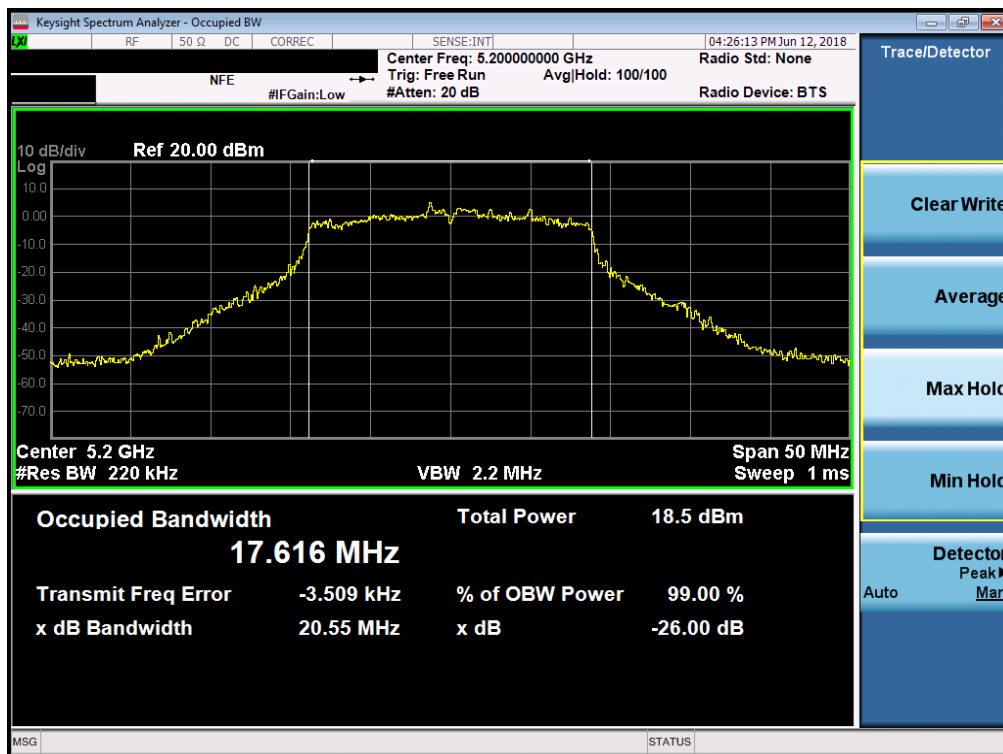
Plot 7-65. 6dB Bandwidth Plot (20MHz BW 802.11n (UNII Band 3) – Ch. 157)
