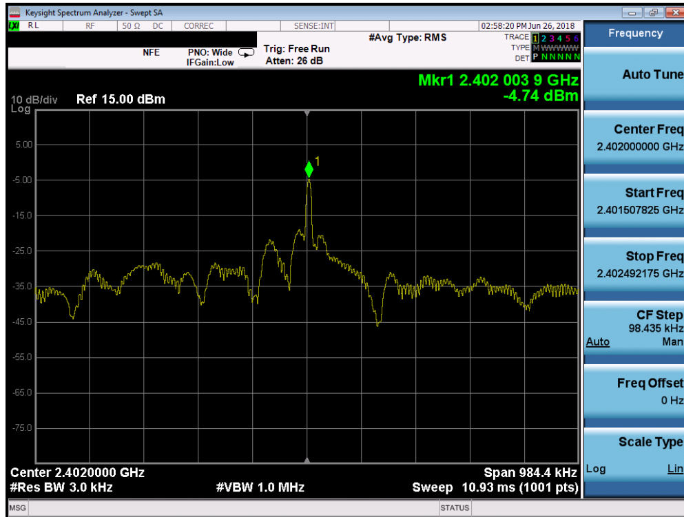
Plot 7-16. Power Spectral Density Plot (Bluetooth (LE), 2Mbps – Ch. 0)
