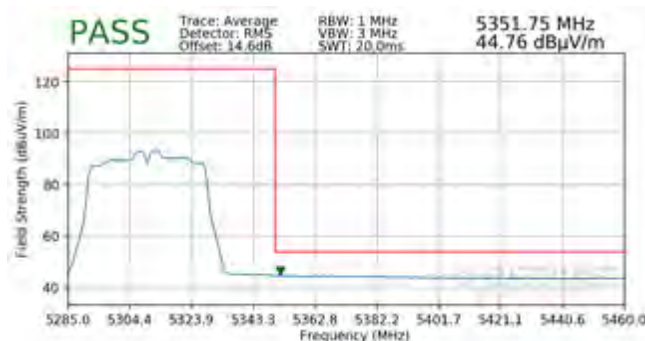
Plot 7-180. Radiated Upper Band Edge Plot SISO ANT1 (Average – UNII Band 2A)
