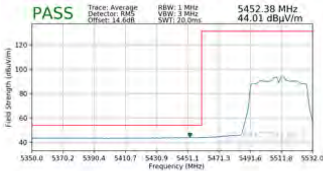
Plot 7-182. Radiated Lower Band Edge Plot SISO ANT1 (Average – UNII Band 2C)
