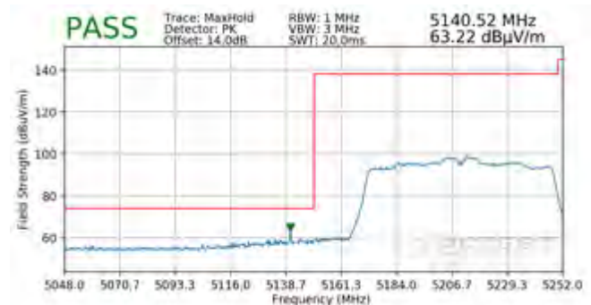
Plot 7-186. Radiated Lower Band Edge Plot SISO ANT1 (Peak – UNII Band 1)
