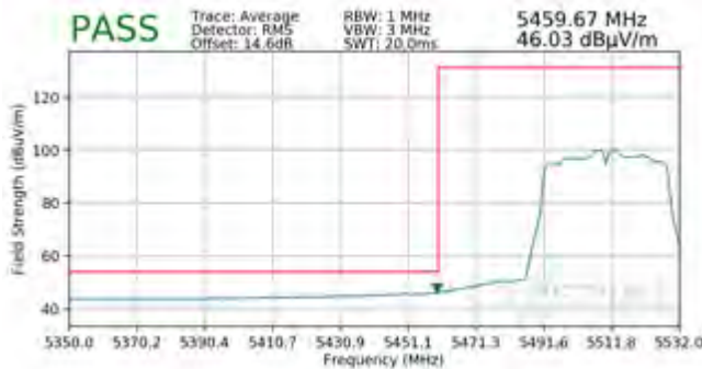
Plot 7-203. Radiated Lower Band Edge Plot SISO ANT2 (Average – UNII Band 2C)
