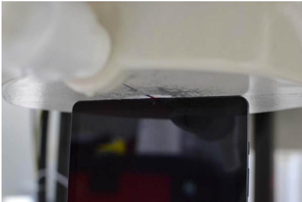
SAR Test Setup Photo 4: Top at 0.0 mm
