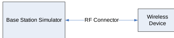
Figure 8-2 Power Measurement Setup
