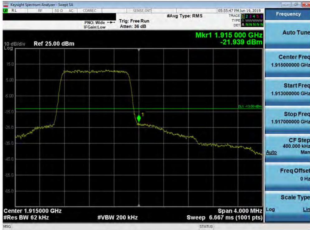
Plot 7-198. Upper Band Edge Plot (Band 25 - 1.4MHz QPSK - Full RB Configuration)
