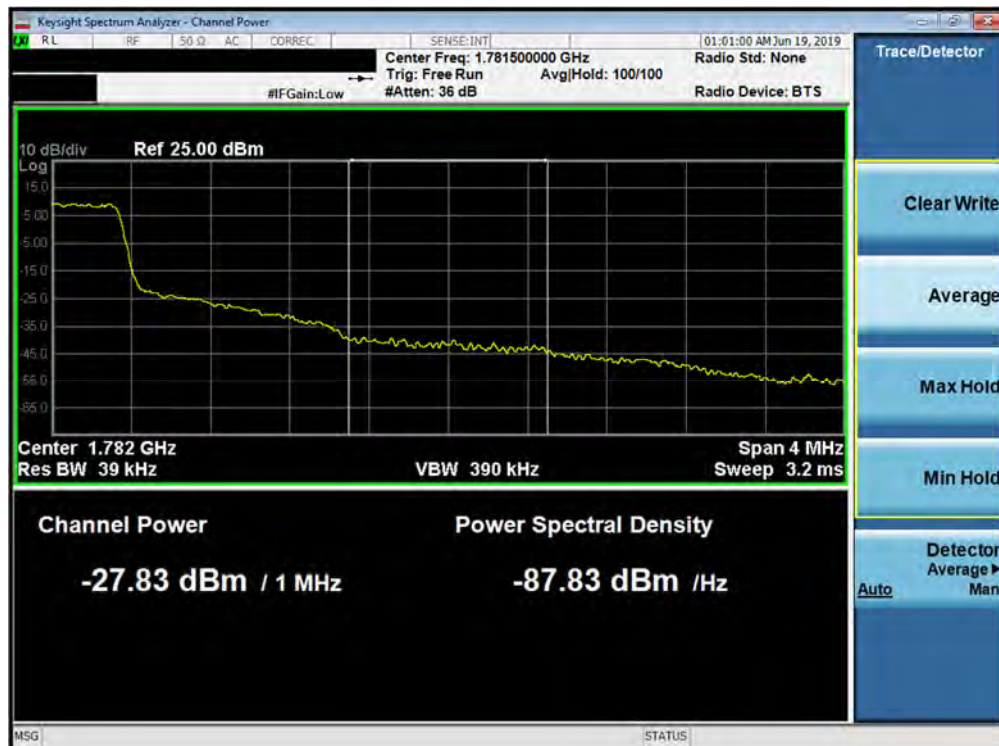
Plot 7-163. Upper Extended Band Edge Plot (Band 66 - 1.4MHz QPSK - Full RB Configuration)
