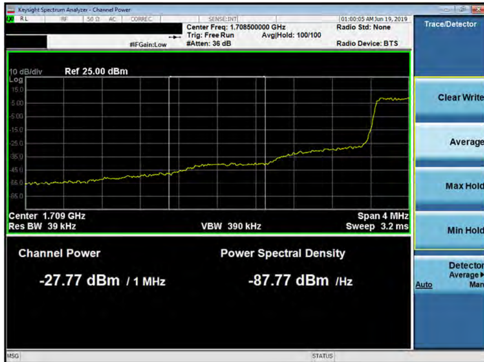
Plot 7-159. Lower Extended Band Edge Plot (Band 66/4 - 1.4MHz QPSK - Full RB Configuration)
