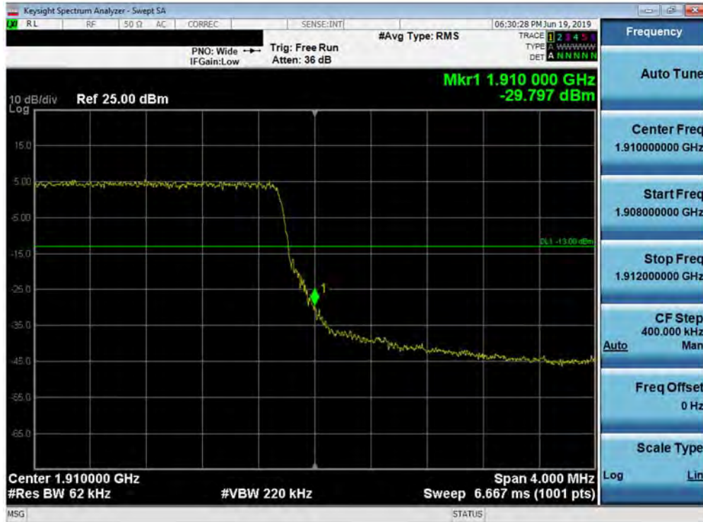
Plot 7-208. Upper Band Edge Plot (Band 2 - 5.0MHz QPSK - Full RB Configuration)
