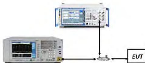
Figure 7-4. Test Instrument & Measurement Setup
