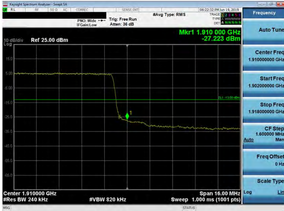
Plot 7-226. Upper Band Edge Plot (Band 2 - 20.0MHz QPSK - Full RB Configuration)
