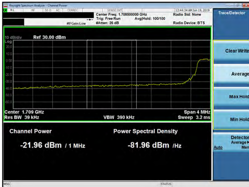
Plot 7-171. Lower Extended Band Edge Plot (Band 66/4 - 5.0MHz QPSK - Full RB Configuration)
