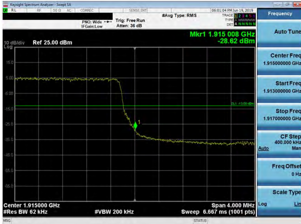
Plot 7-210. Upper Band Edge Plot (Band 25 - 5.0MHz QPSK - Full RB Configuration)
