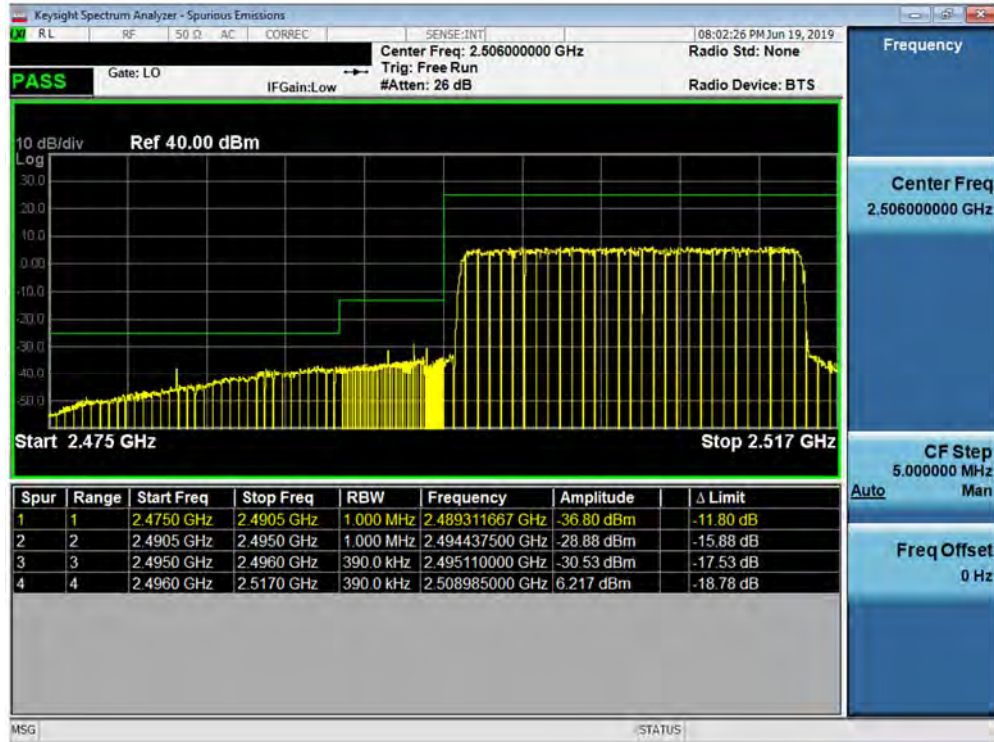
Plot 7-236. Lower ACP Plot (Band 41 - 20.0MHz QPSK - Full RB Configuration)
