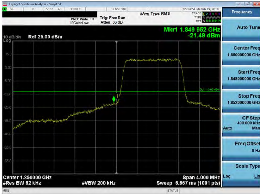
Plot 7-194. Lower Band Edge Plot (Band 25/2 - 1.4MHz QPSK - Full RB Configuration)
