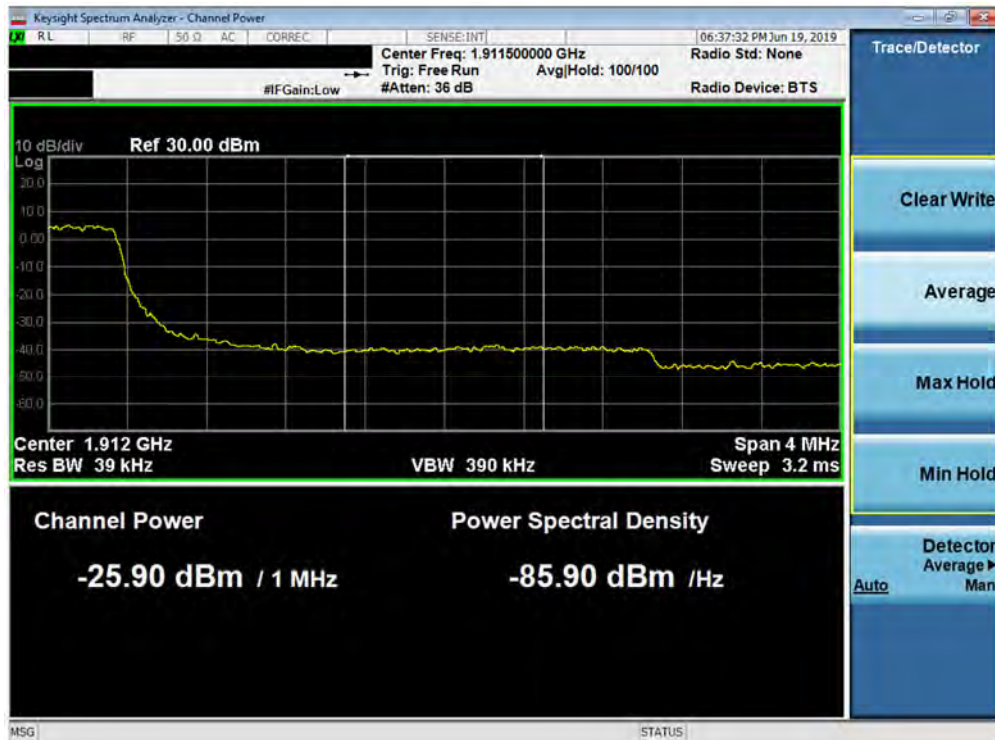
Plot 7-203. Upper Extended Band Edge Plot (Band 2 - 3.0MHz QPSK - Full RB Configuration)
