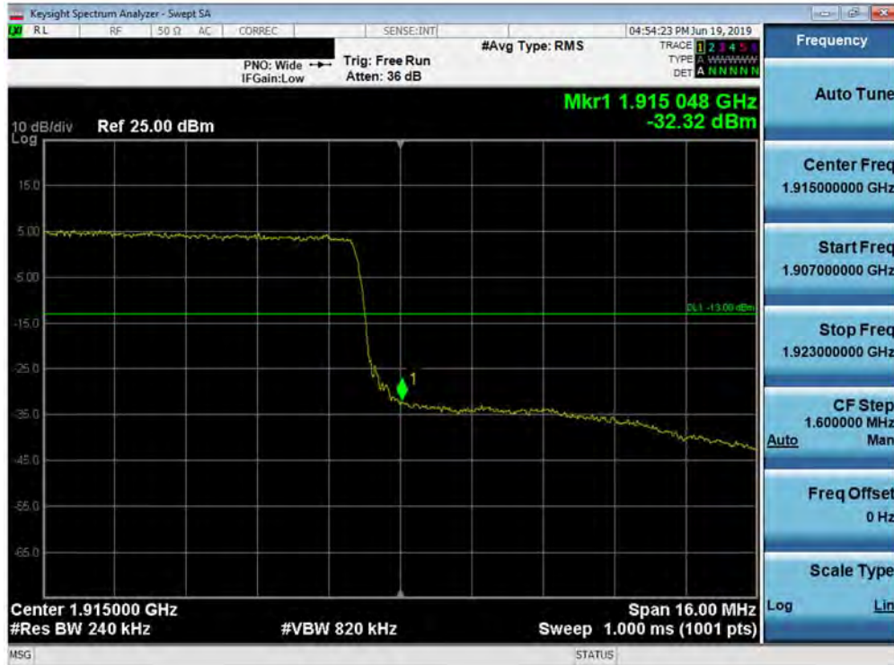
Plot 7-228. Upper Band Edge Plot (Band 25 - 20.0MHz QPSK - Full RB Configuration)
