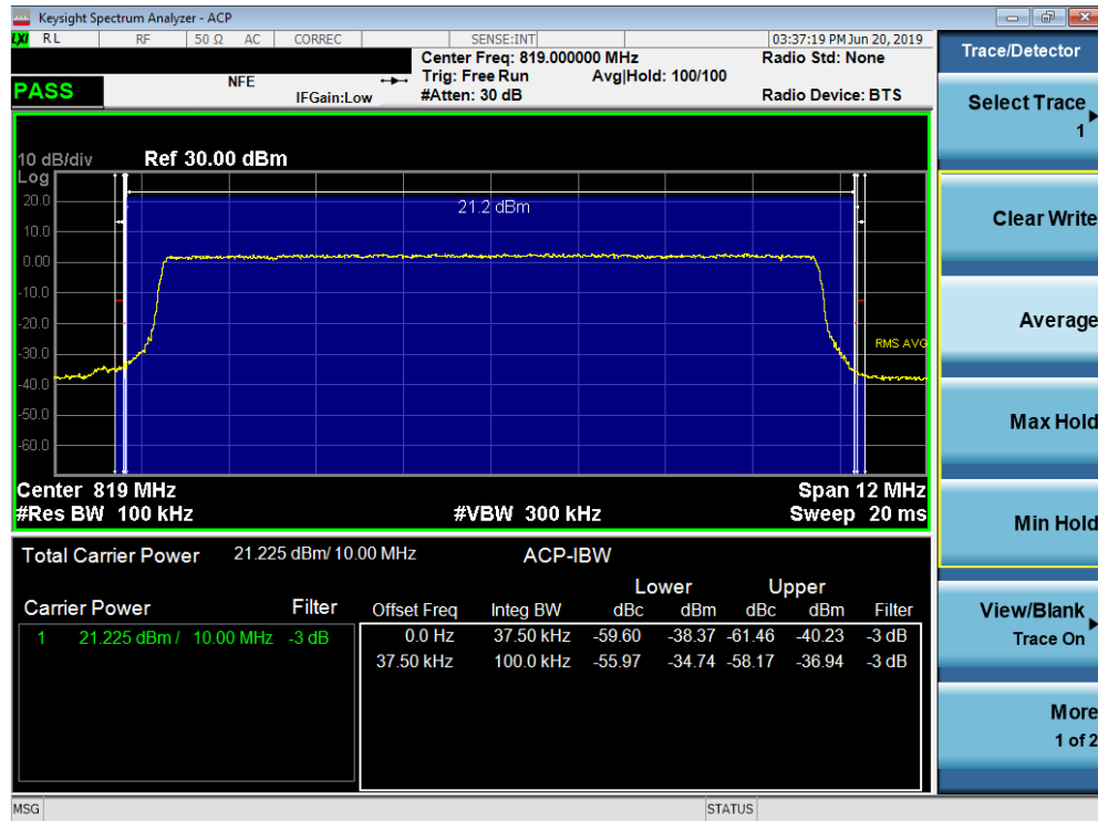
Plot 7-28. Channel Edge Plot (LTE Band 26, 10MHz QPSK – RB Size 50)
