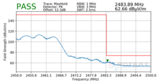
Plot 7-141. Radiated Restricted Upper Band Edge Measurement MIMO (Peak)
