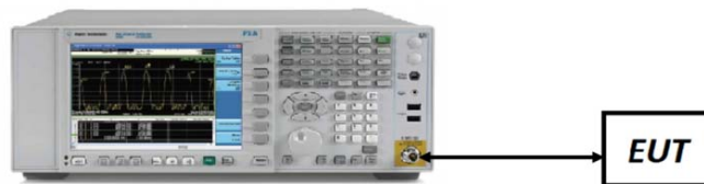
Figure 7-1. Test Instrument & Measurement Setup
