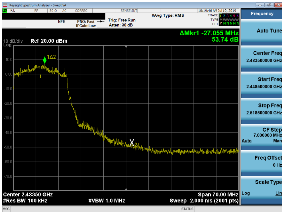
Plot 7-67. Band Edge Plot SISO ANT2 (802.11g – Ch. 10)
