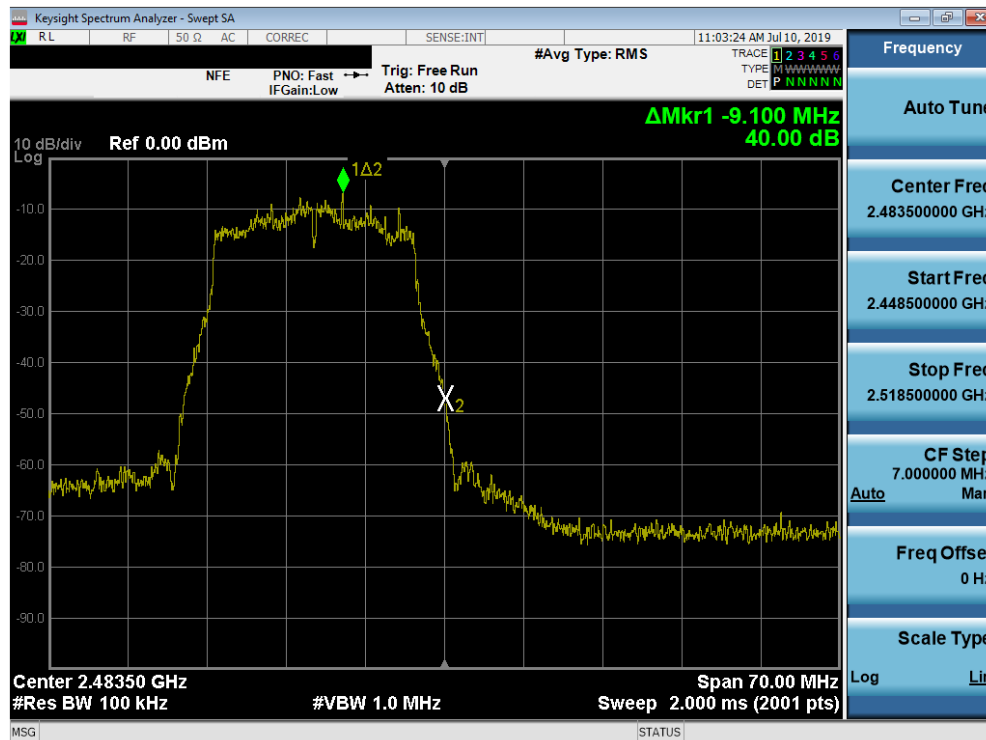
Plot 7-58. Band Edge Plot SISO ANT1 (802.11n (2.4GHz) – Ch. 13)
