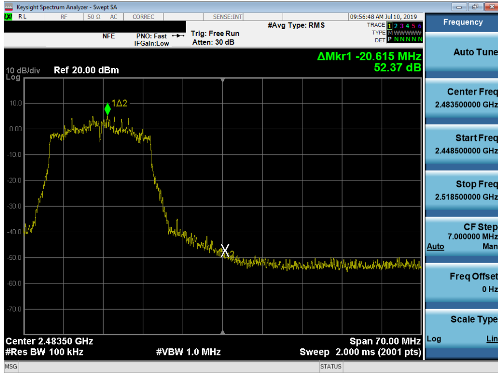
Plot 7-77. Band Edge Plot SISO ANT2 (802.11n (2.4GHz) – Ch. 11)
