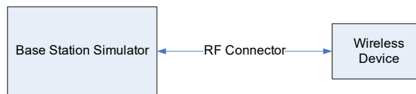
Figure 8-2 Power Measurement Setup
