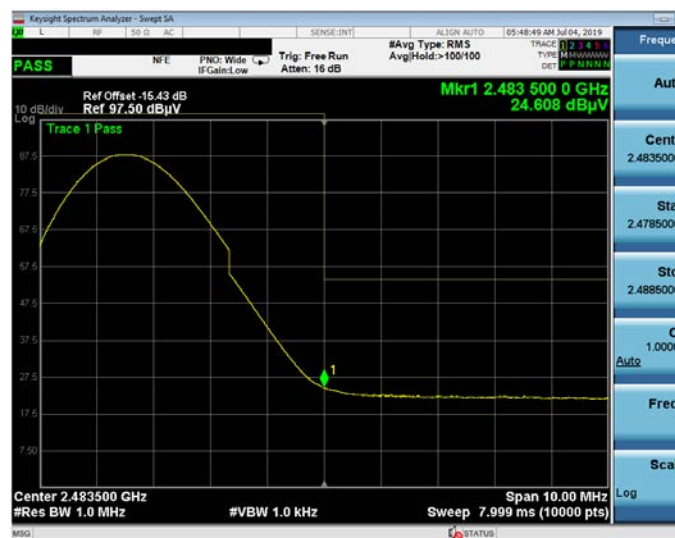
Plot 7-46. Radiated Restricted Upper Band Edge Measurement (Average)
