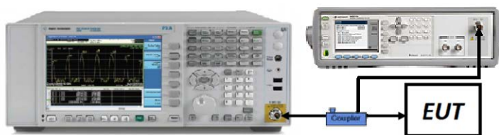
Figure 7-2. Test Instrument & Measurement Setup
