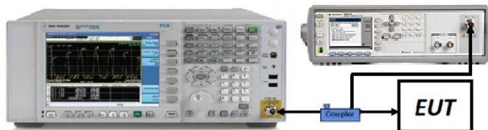
Figure 7-1. Test Instrument & Measurement Setup
