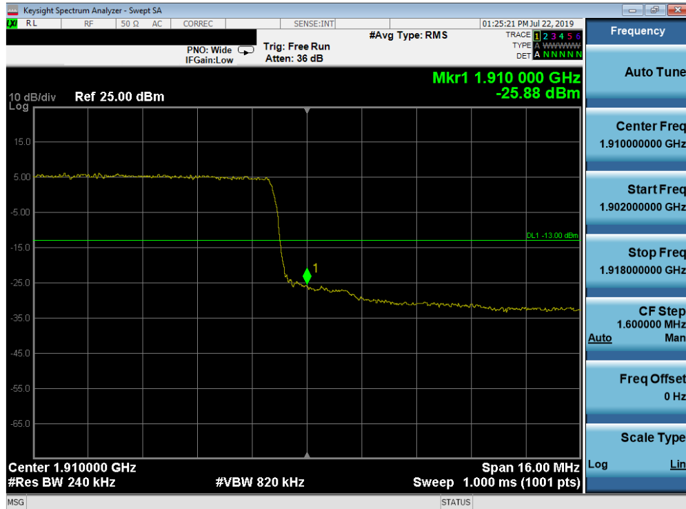
Plot 7-180. Upper Band Edge Plot (Band 2 - 20.0MHz QPSK - Full RB Configuration)
