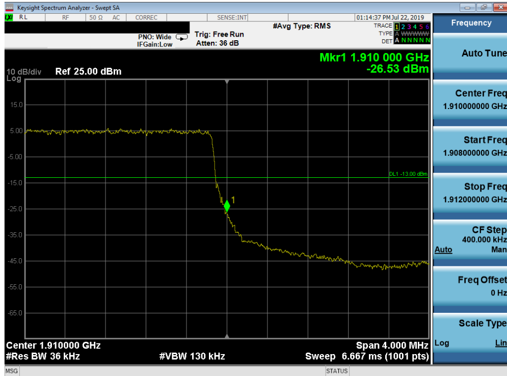
Plot 7-164. Upper Band Edge Plot (Band 2 - 3.0MHz QPSK - Full RB Configuration)
