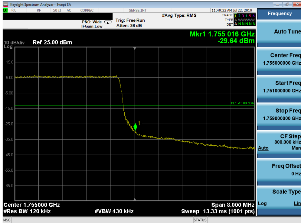
Plot 7-142. Upper Band Edge Plot (Band 4 - 10.0MHz QPSK - Full RB Configuration)
