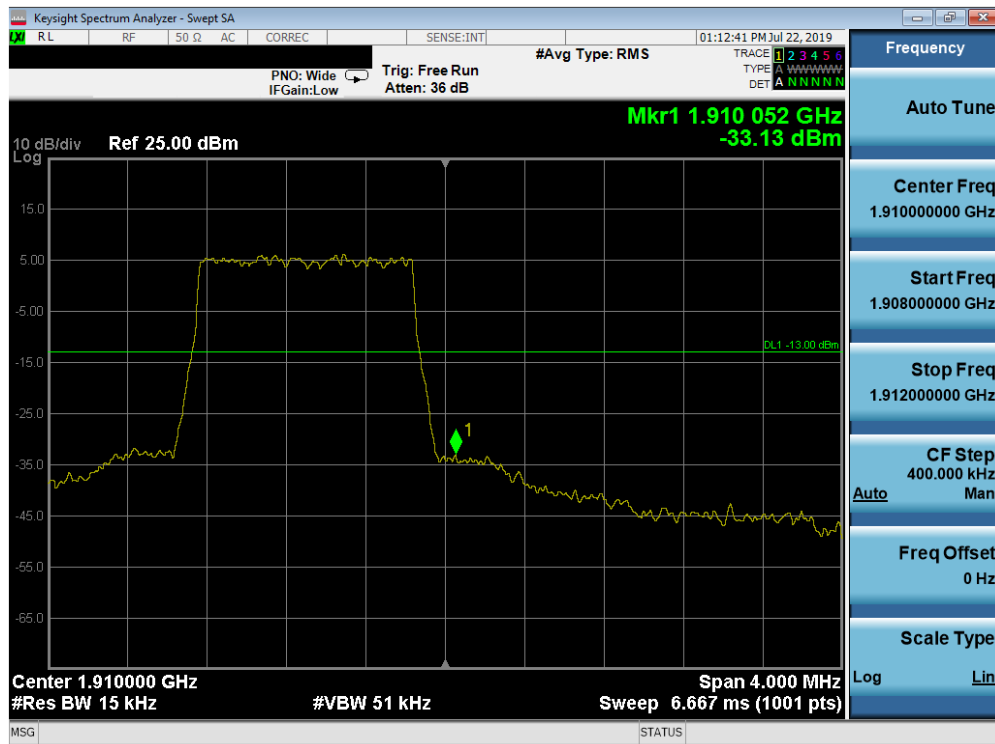
Plot 7-160. Upper Band Edge Plot (Band 2 - 1.4MHz QPSK - Full RB Configuration)
