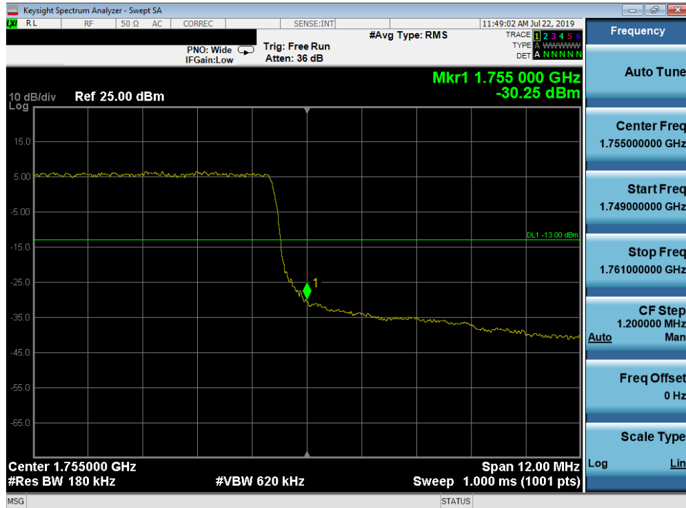
Plot 7-148. Upper Band Edge Plot (Band 4 - 15.0MHz QPSK - Full RB Configuration)
