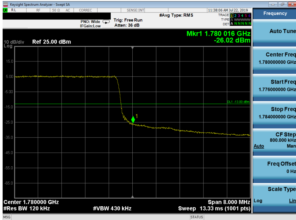
Plot 7-144. Upper Band Edge Plot (Band 66 - 10.0MHz QPSK - Full RB Configuration)
