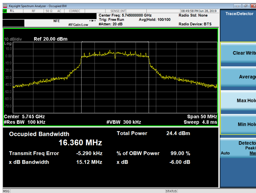
Plot 7-59. 6dB Bandwidth Plot SISO ANT1 (802.11a (UNII Band 3) – Ch. 149)
