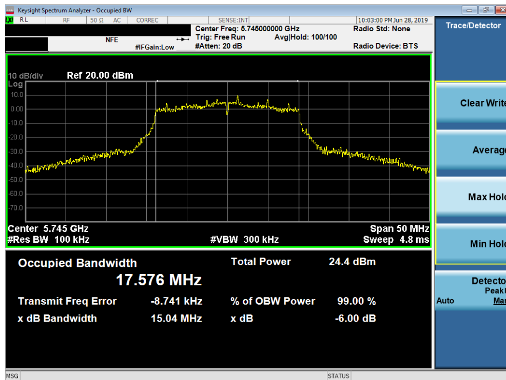
Plot 7-71. 6dB Bandwidth Plot SISO ANT2 (20MHz BW 802.11n (UNII Band 3) – Ch. 149)
