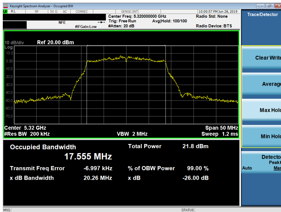
Plot 7-44. 26dB Bandwidth Plot SISO ANT2 (20MHz BW 802.11n (UNII Band 2A) – Ch. 64)
