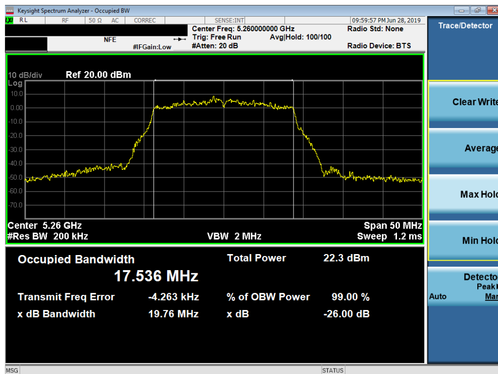
Plot 7-42. 26dB Bandwidth Plot SISO ANT2 (20MHz BW 802.11n (UNII Band 2A) – Ch. 52)
