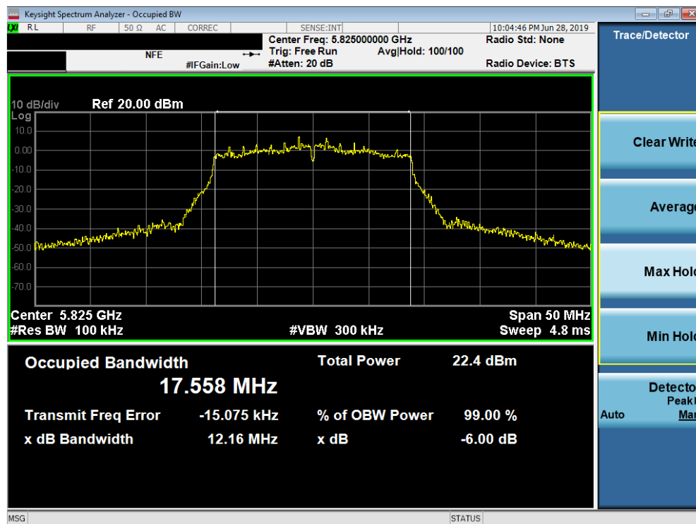
Plot 7-73. 6dB Bandwidth Plot SISO ANT2 (20MHz BW 802.11n (UNII Band 3) – Ch. 165)
