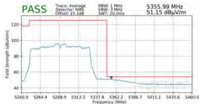
Plot 7-229. Radiated Upper Band Edge Plot MIMO (Average – UNII Band 2A)
