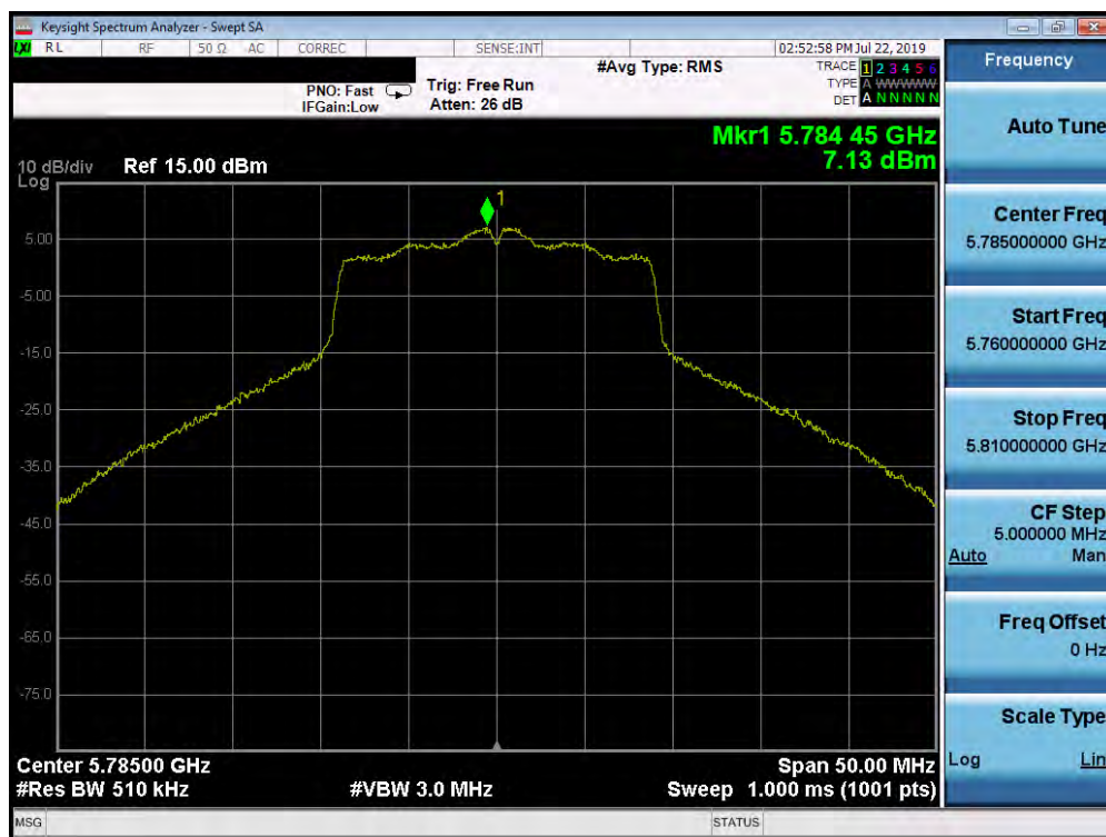
Plot 7-148. Power Spectral Density Plot SISO ANT2 (20MHz BW 802.11n (UNII Band 3) – Ch. 157)
