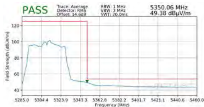
Plot 7-222. Radiated Upper Band Edge Plot MIMO (Average – UNII Band 2A)
