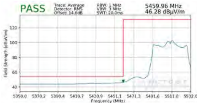
Plot 7-224. Radiated Lower Band Edge Plot MIMO (Average – UNII Band 2C)
