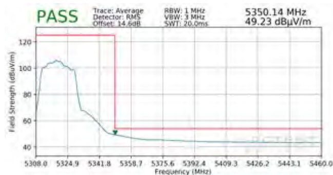
Plot 7-215. Radiated Upper Band Edge Plot MIMO (Average – UNII Band 2A)
