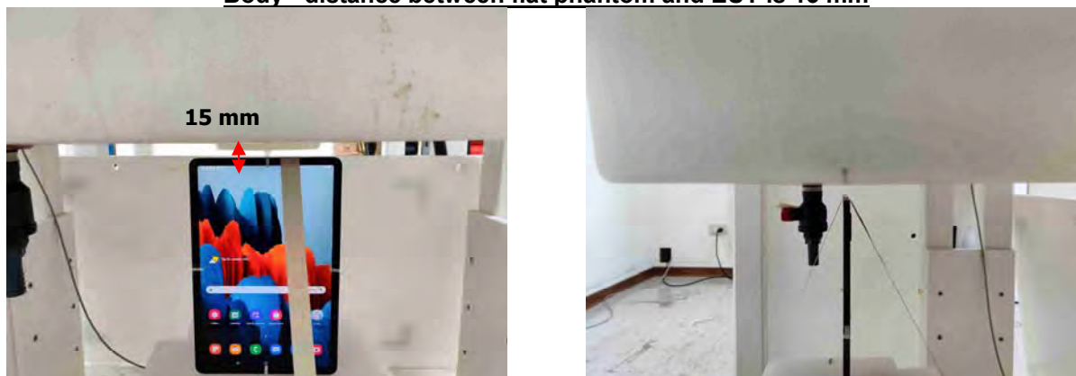
Fig.17 EUT Top side to flat phantom
