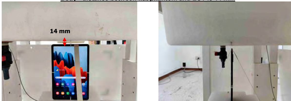
Fig.16 EUT Top side to flat phantom
