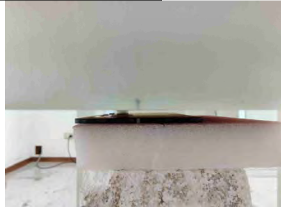
Fig.12 EUT Back side to flat phantom
