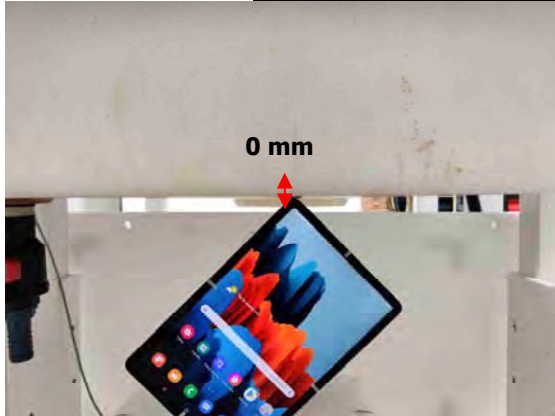
Fig.9 EUT Left corner side to flat phantom
