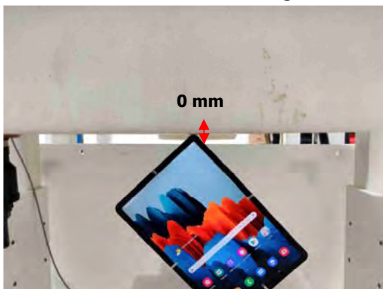
Fig.8 EUT Right corner side to flat phantom
