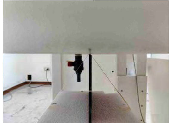
Fig.6 EUT Right side to flat phantom
