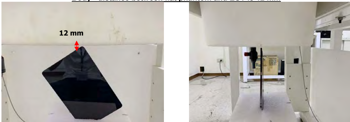
Fig.15 EUT Right corner side to flat phantom
