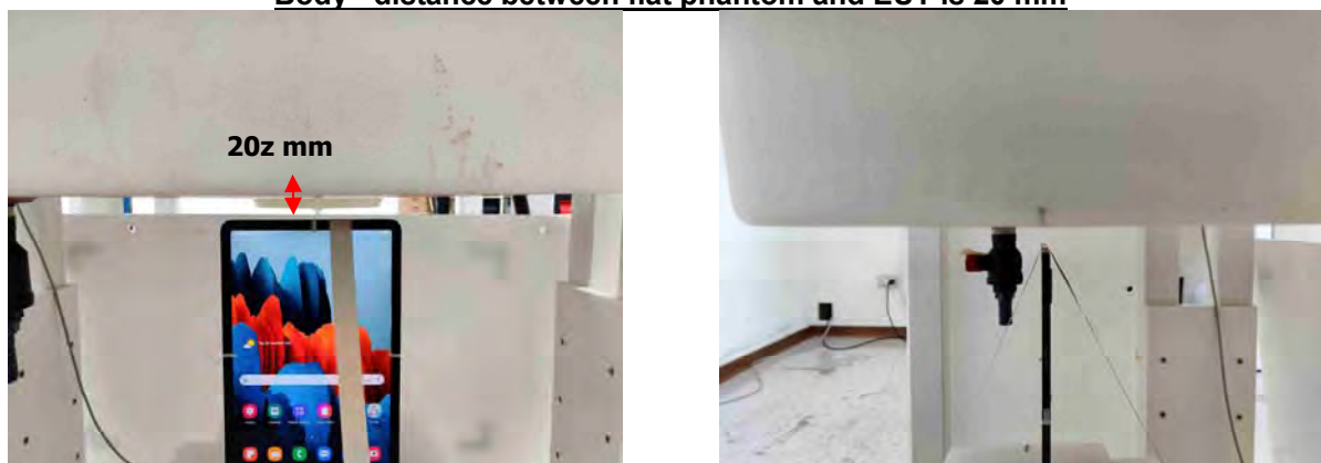
Fig.18 EUT Top side to flat phantom
