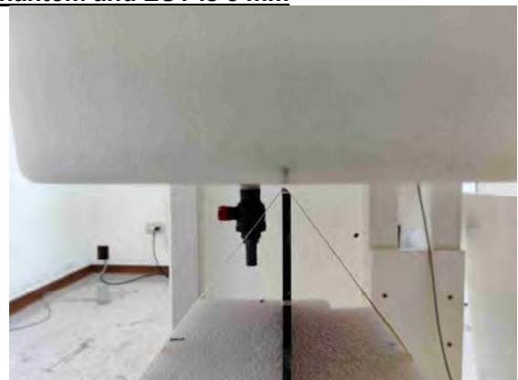
Fig.11 EUT Right side to flat phantom
