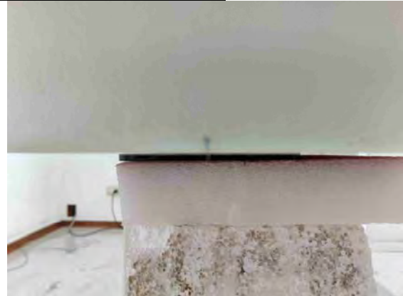
Fig.3 EUT Back side to flat phantom
