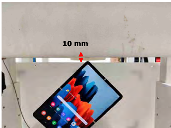
Fig.13 EUT Left corner side to flat phantom
