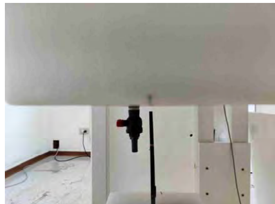
Fig.13 EUT Left corner side to flat phantom
