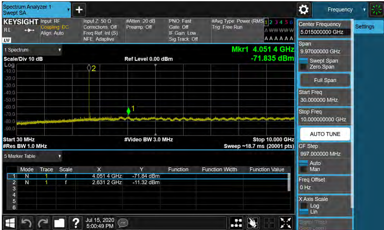
Sub6 n41. Conducted Spurious Plot 1 (60 MHz Ch.531996 BPSK RB 1, Offset 0)
