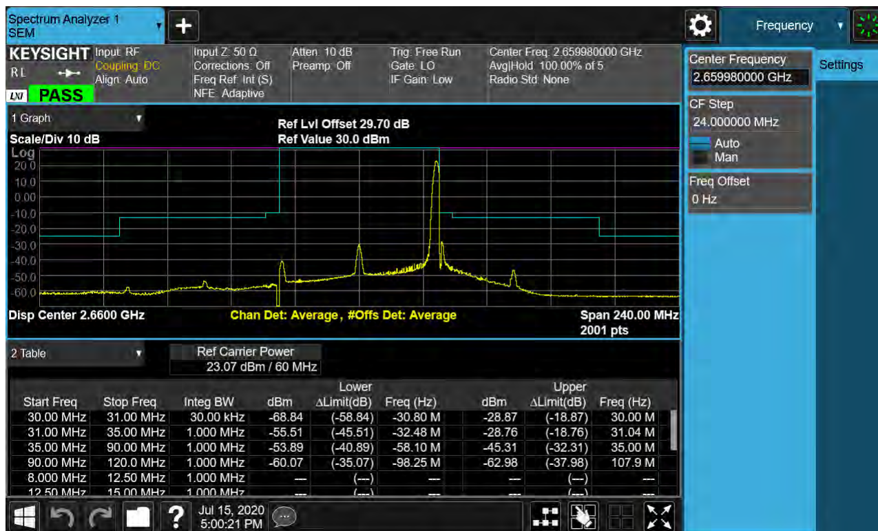
Sub6 n41. High Channel Edge Plot (60 MHz Ch.531996 BPSK RB 1)
