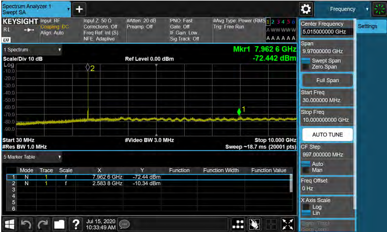
Sub6 n41. Conducted Spurious Plot 1 (20 MHz Ch.518598 BPSK RB 1, Offset 0)
