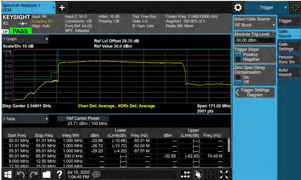
Sub6 n41. Low Channel Edge Plot (100 MHz Ch.509202 BPSK RB 25, Offset 0)-1
