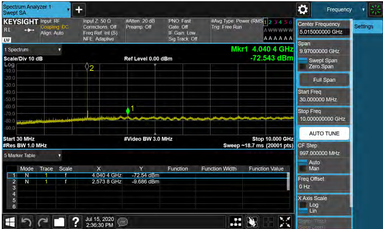
Sub6 n41. Conducted Spurious Plot 1 (40 MHz Ch.518598 BPSK RB 1, Offset 0)
