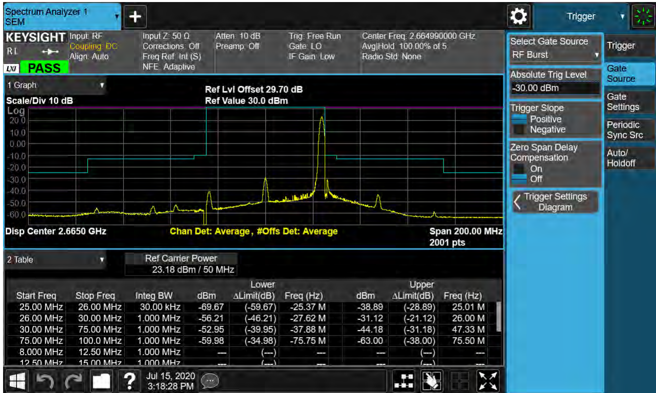
Sub6 n41. High Channel Edge Plot (50 MHz Ch.532998 BPSK RB 1)
