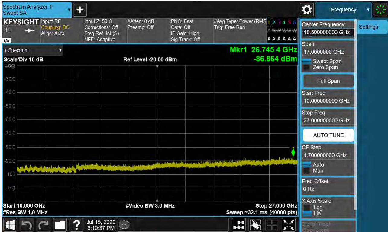
Sub6 n41. Conducted Spurious Plot 2 (80 MHz Ch.507204 BPSK RB 1, Offset 0)
