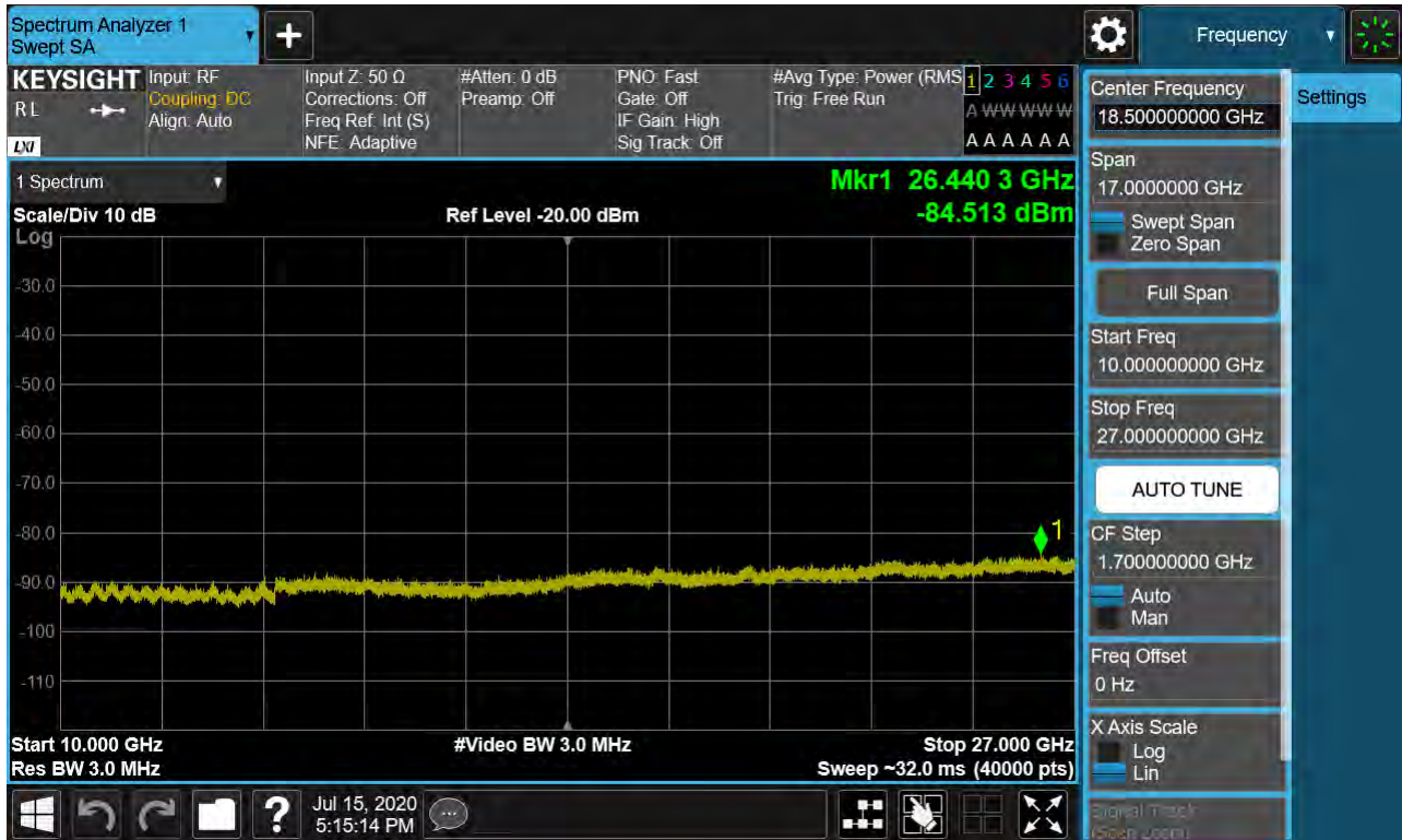
Sub6 n41. Conducted Spurious Plot 2 (80 MHz Ch. 518598 BPSK RB 1, Offset 0)
