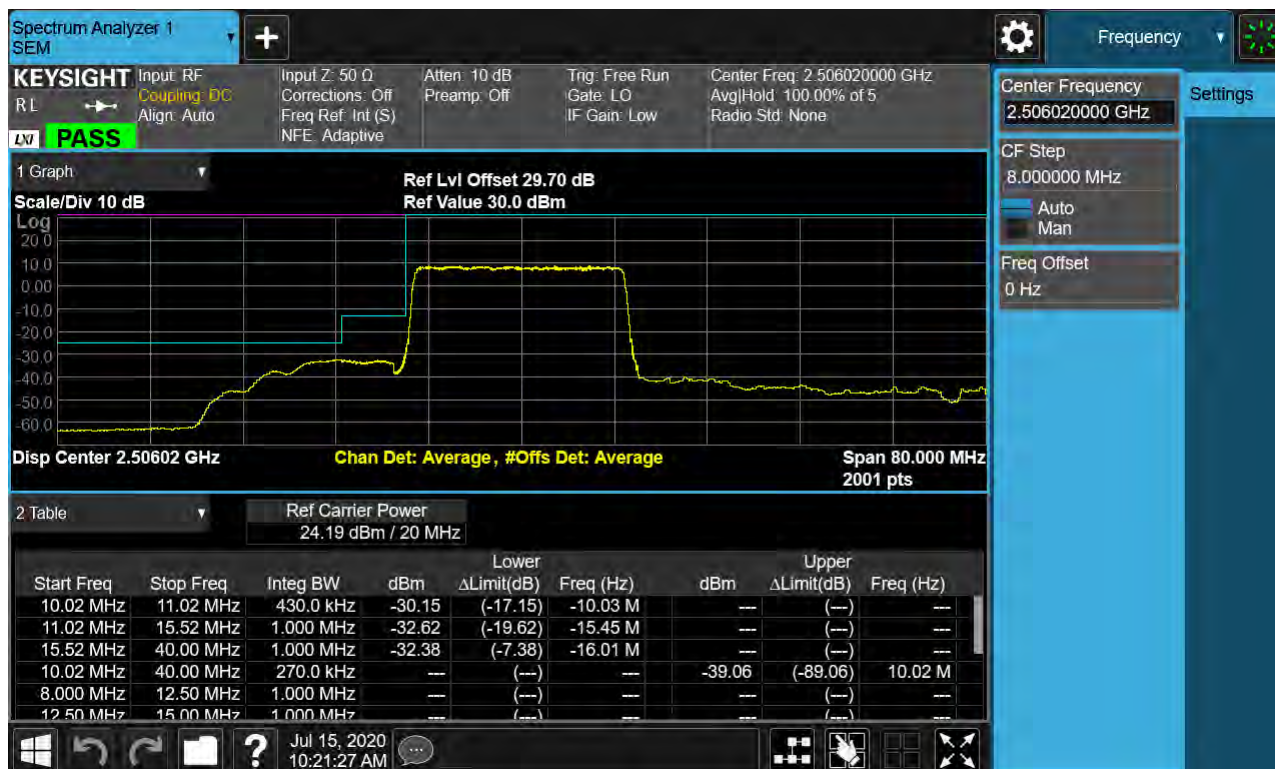
Sub6 n41. Low Channel Edge Plot (20 MHz Ch.501204 BPSK RB 25, Offset 0)-1
