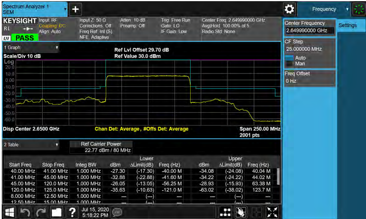
Sub6 n41. High Channel Edge Plot (80 MHz Ch.529998 BPSK_RB25_Offset 0)
