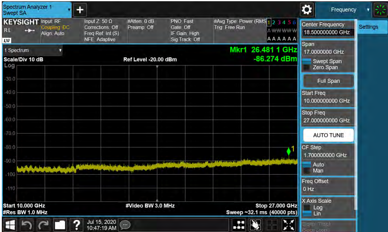
Sub6 n41. Conducted Spurious Plot 2 (20 MHz Ch.535998 BPSK RB 1, Offset 0)
