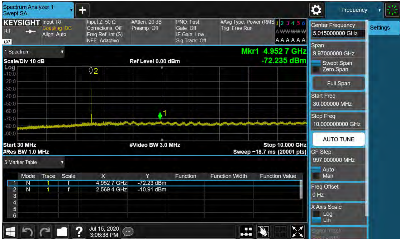
Sub6 n41. Conducted Spurious Plot 1 (50 MHz Ch.518598 BPSK RB 1, Offset 0)
