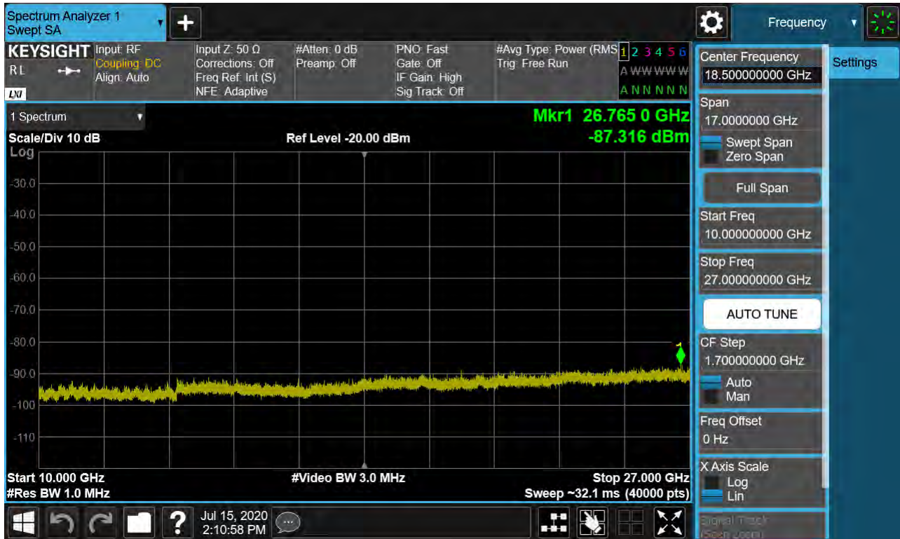
Sub6 n41. Conducted Spurious Plot 2 (40 MHz Ch.503202 BPSK RB 1, Offset 0)
