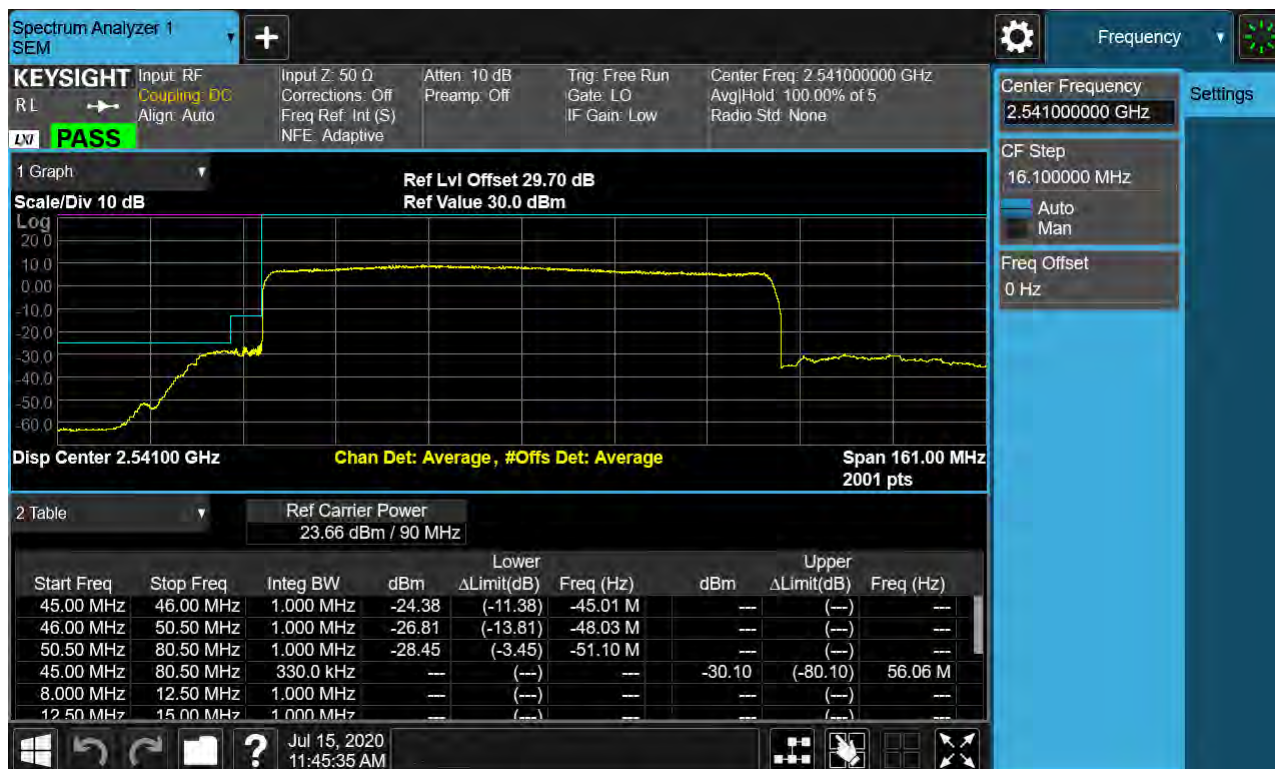
Sub6 n41. Low Channel Edge Plot (90 MHz Ch.508200 BPSK RB 25, Offset 0)-1
