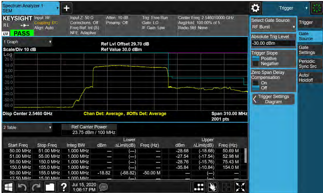
Sub6 n41. Low Channel Edge Plot (100 MHz Ch.509202 BPSK_RB25_Offset 0)-2
