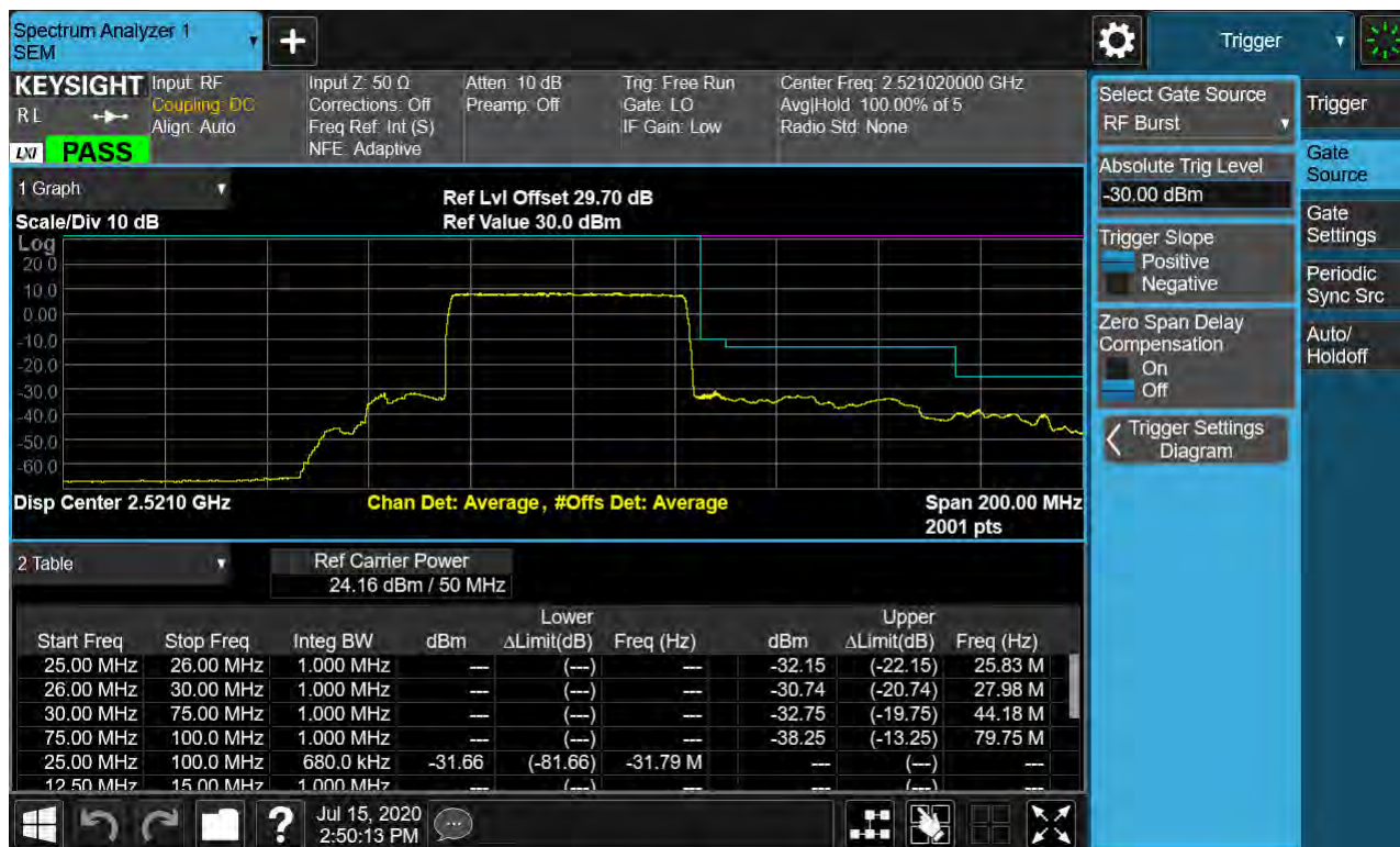
Sub6 n41. Low Channel Edge Plot (50 MHz Ch.504204 BPSK_RB25_Offset 0)-2
