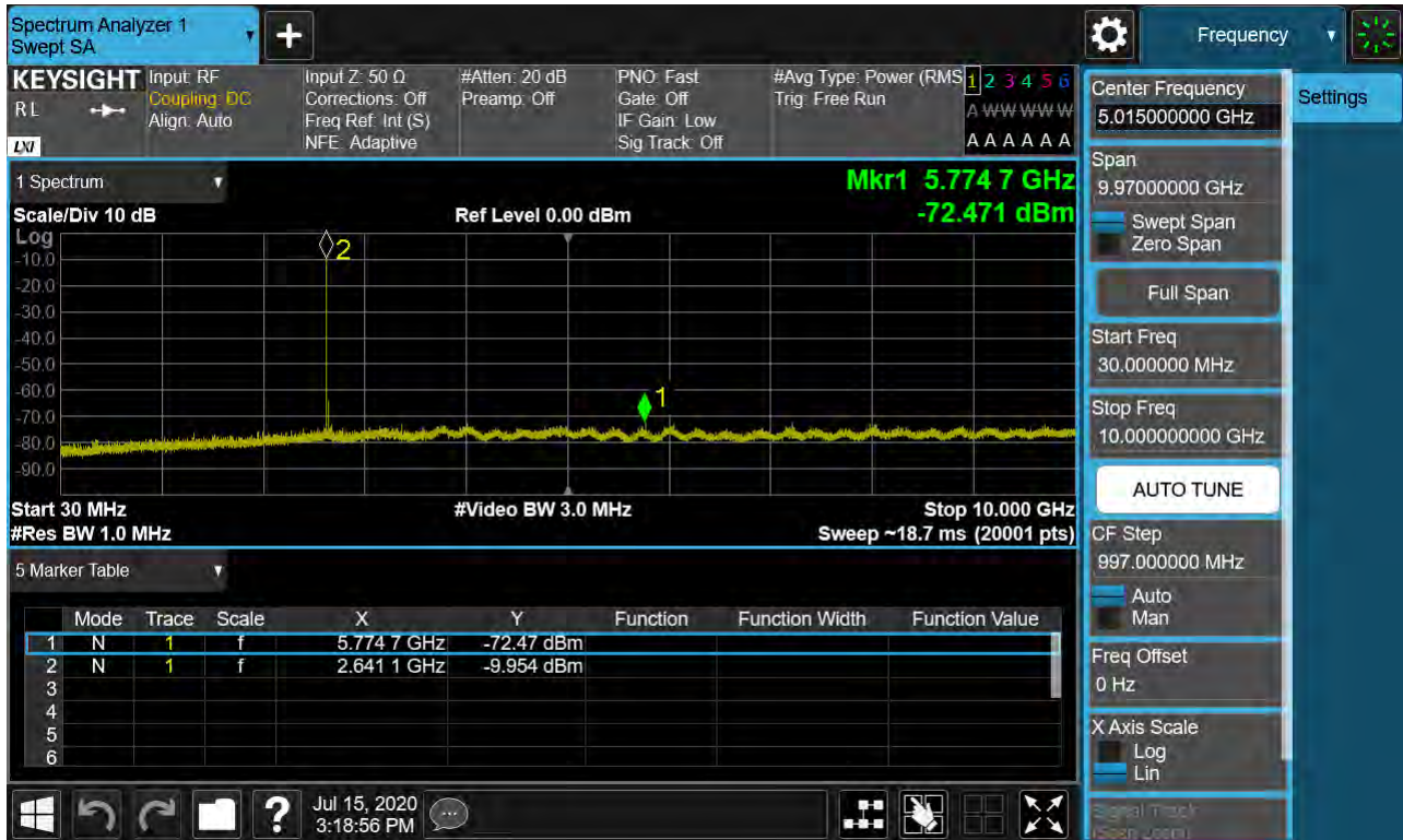
Sub6 n41. Conducted Spurious Plot 1 (50 MHz Ch.532998 BPSK RB 1, Offset 0)
