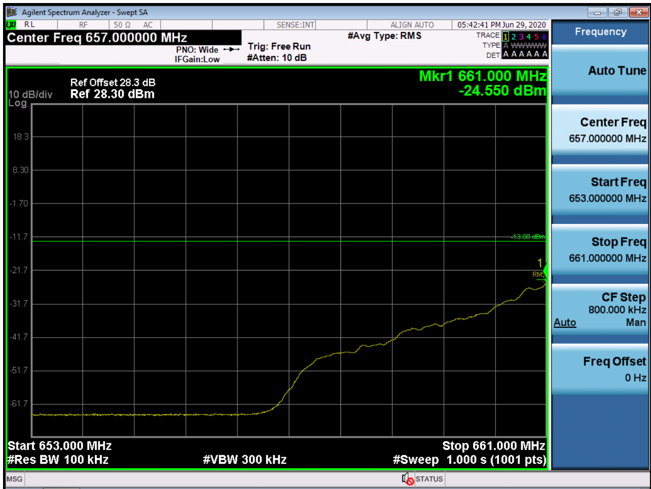
Sub6 n71. Lower Extended Band Edge Plot (5M BW Ch.133100 BPSK_RB6_0)
