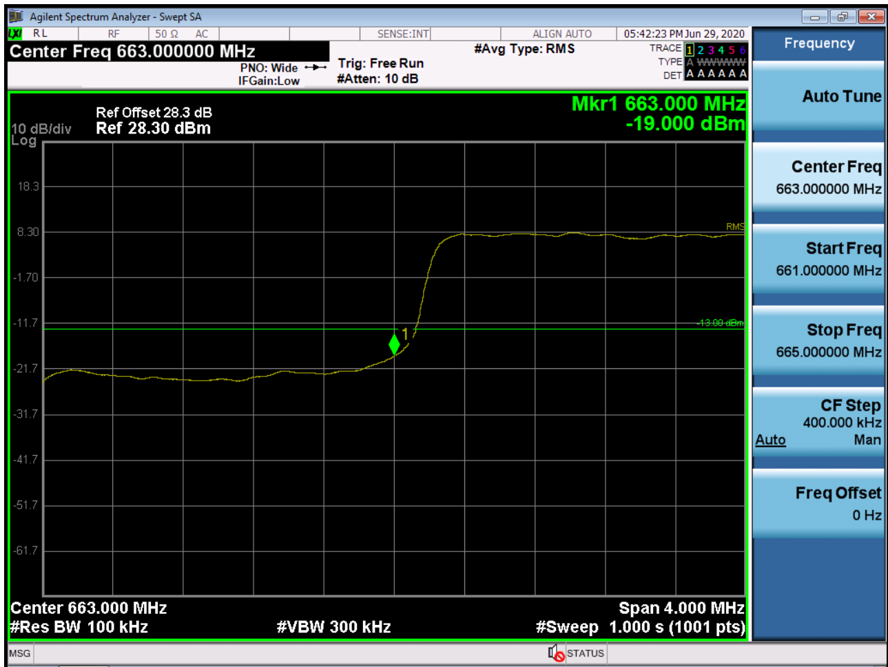
Sub6 n71. Lower Band Edge Plot (5M BW Ch.133100 BPSK_RB6_Offset 0)
