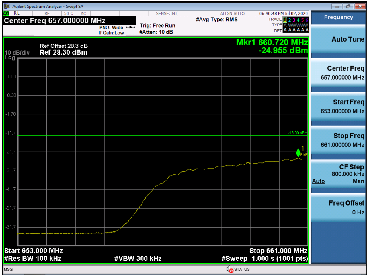
Sub6 n71. Lower Extended Band Edge Plot (20M BW Ch.134600 BPSK_RB50_0)
