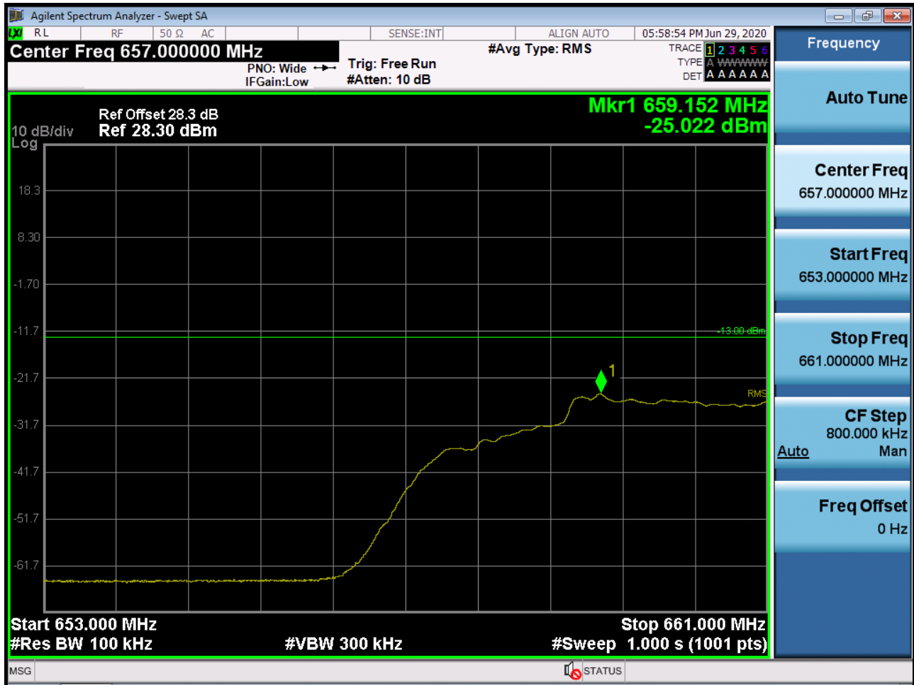
Sub6 n71. Lower Extended Band Edge Plot (10M BW Ch.133600 BPSK_RB15_0)
