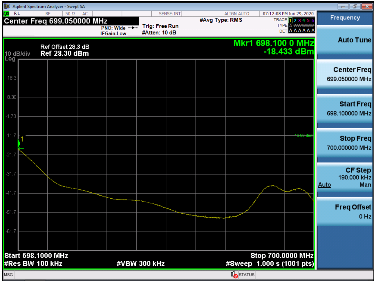
Sub6 n71. Upper Band Edge Plot (5M BW Ch.139100 BPSK_RB1_Offset 5)_2
