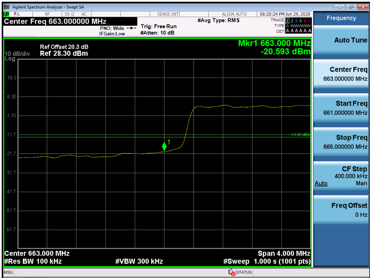
Sub6 n71. Lower Band Edge Plot (15M BW Ch.134100 BPSK_RB25_Offset 0)
