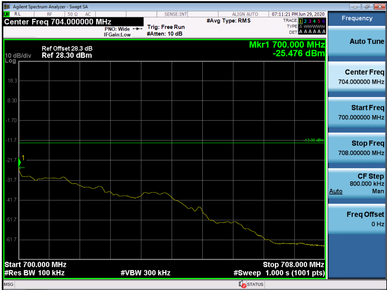
Sub6 n71. Upper Extended Band Edge Plot (5M BW Ch.139100 BPSK_RB6_0)
