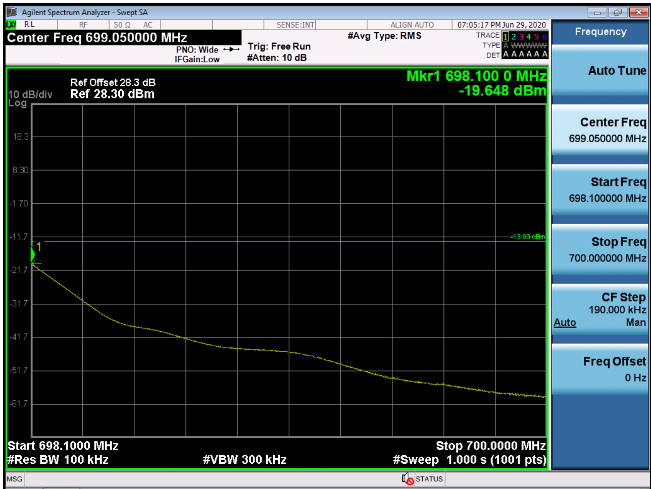
Sub6 n71. Upper Band Edge Plot (10M BW Ch.138600 BPSK_RB1_Offset 14)-2
