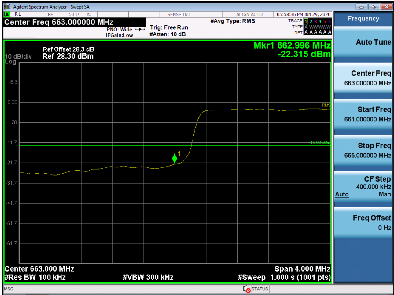
Sub6 n71. Lower Band Edge Plot (10M BW Ch.133600 BPSK_RB15_Offset 0)
