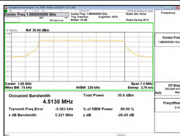
LTE B2 5MHz QPSK Mid Channel RB25-0
