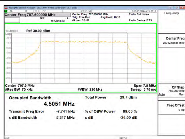
LTE B12 5MHz 16QAM Mid Channel RB25-0
