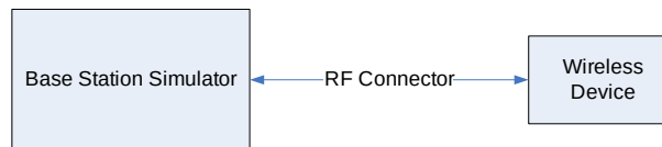
Figure 8-2 Power Measurement Setup
