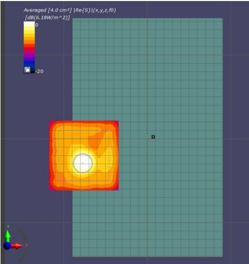
Figure 12-2 4cm 2 psPD distribution measured at input.power.limit of 5.6 dBm on the back surface for n260 beam 24
