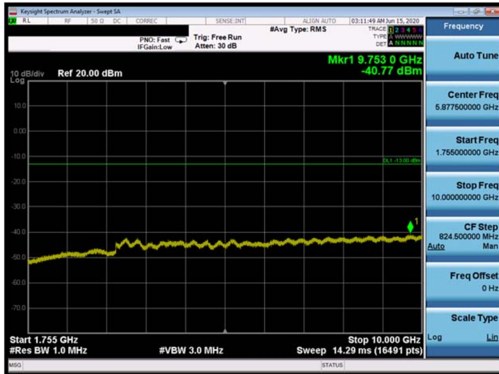
Plot 7-17. Conducted Spurious Plot (AWS WCDMA Mode - Mid Channel)
