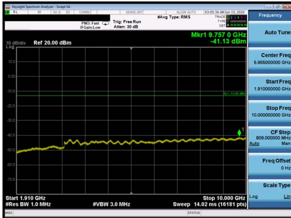
Plot 7-26. Conducted Spurious Plot (PCS WCDMA Mode - Mid Channel)
