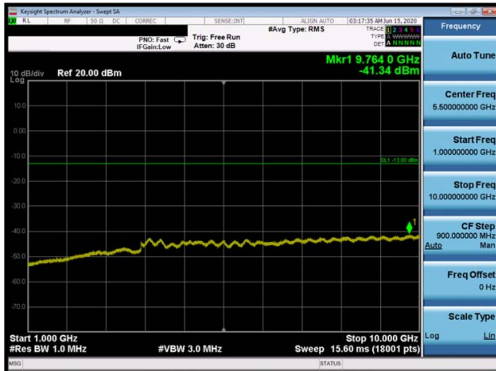
Plot 7-9. Conducted Spurious Plot (Cellular WCDMA Mode - Mid Channel)
