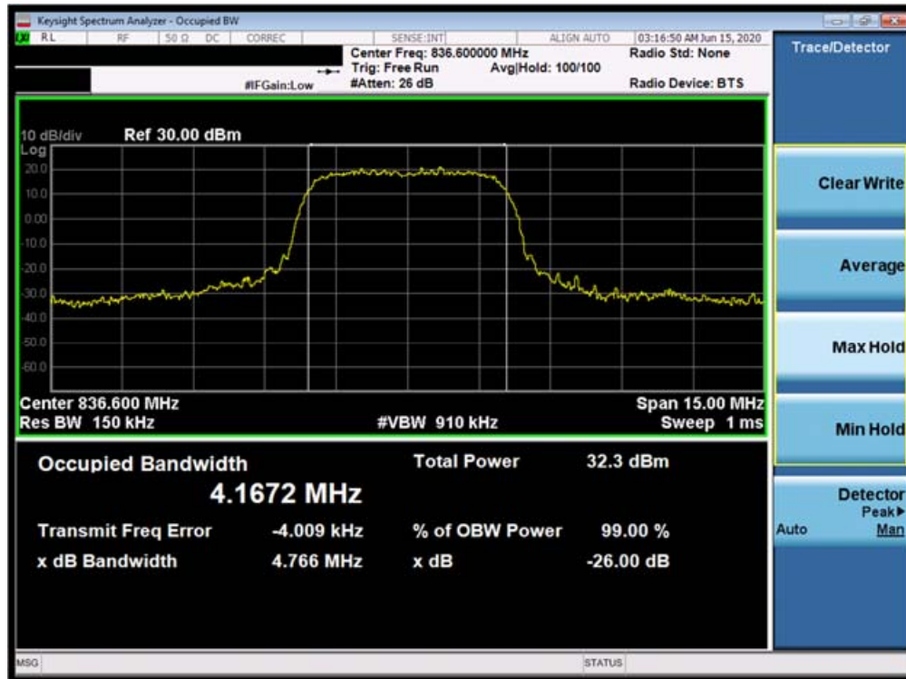
Plot 7-1. Occupied Bandwidth Plot (Cellular WCDMA Mode)
