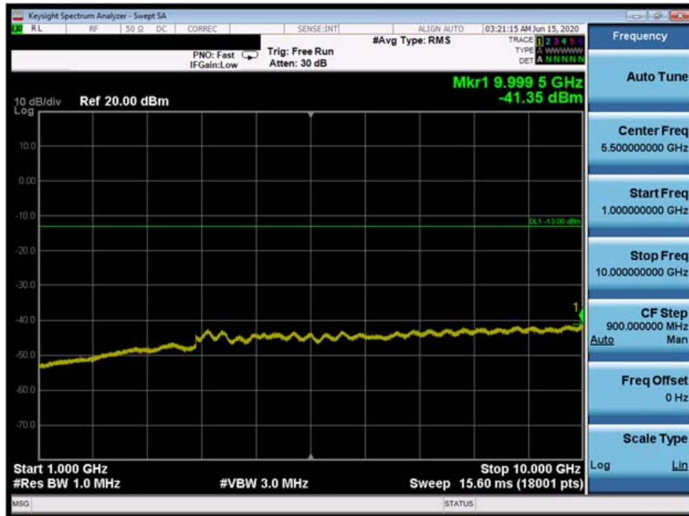
Plot 7-12. Conducted Spurious Plot (Cellular WCDMA Mode - High Channel)
