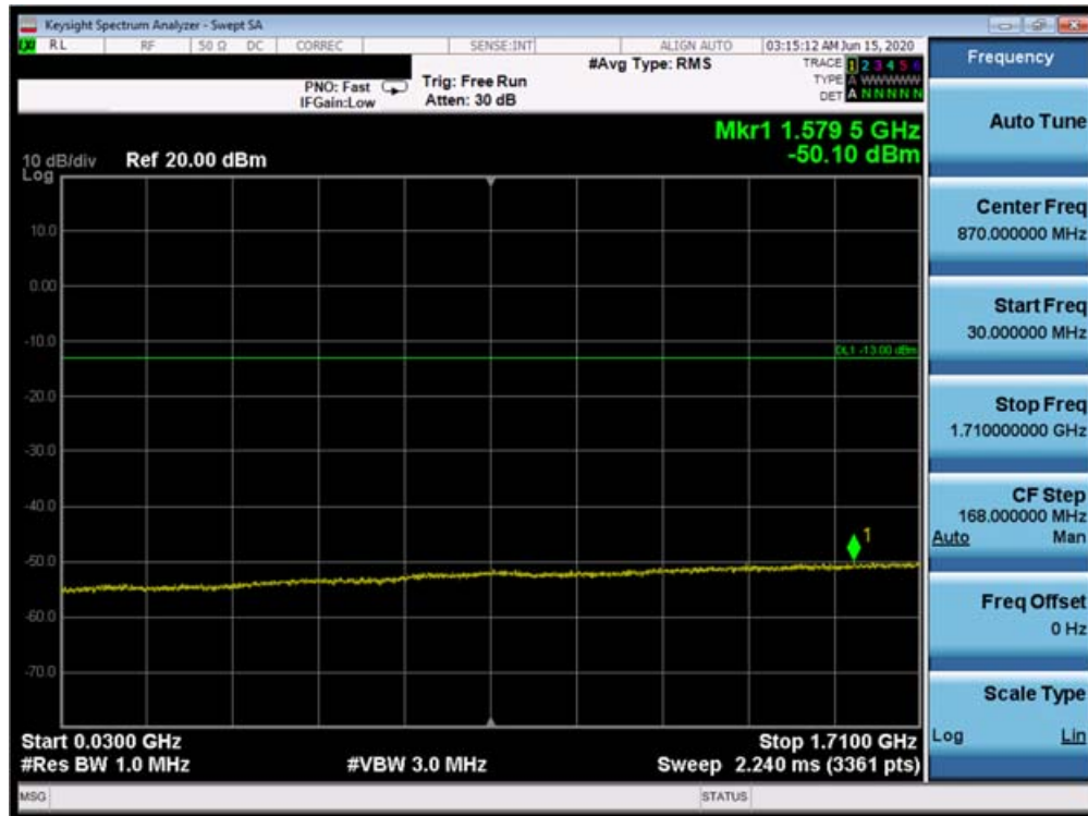
Plot 7-19. Conducted Spurious Plot (AWS WCDMA Mode - High Channel)
