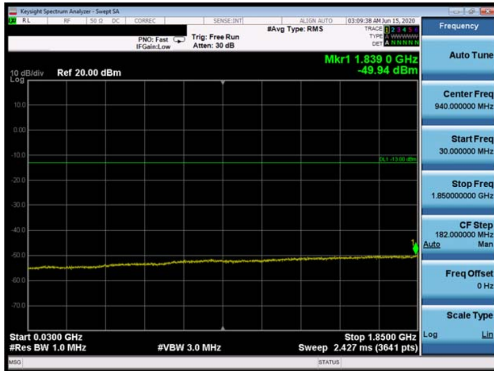
Plot 7-28. Conducted Spurious Plot (PCS WCDMA Mode - High Channel)
