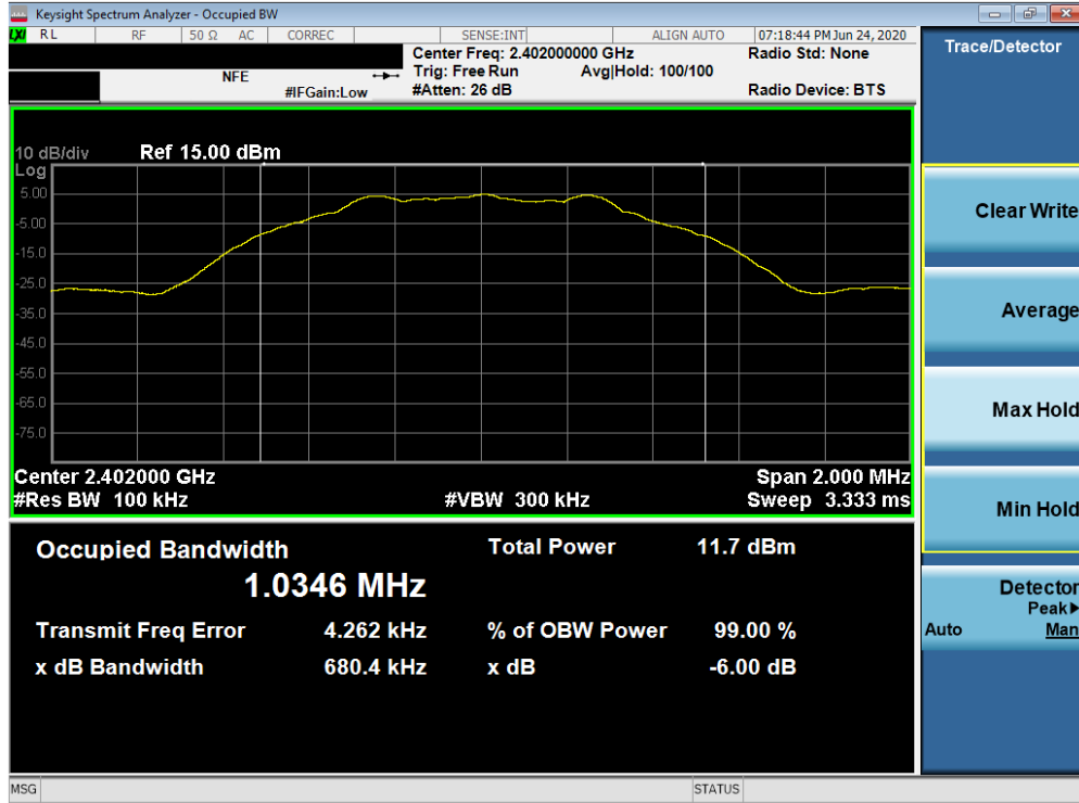
Plot 7-7. 6dB Bandwidth Plot (Bluetooth (LE), 1Mbps – Ch. 0)
