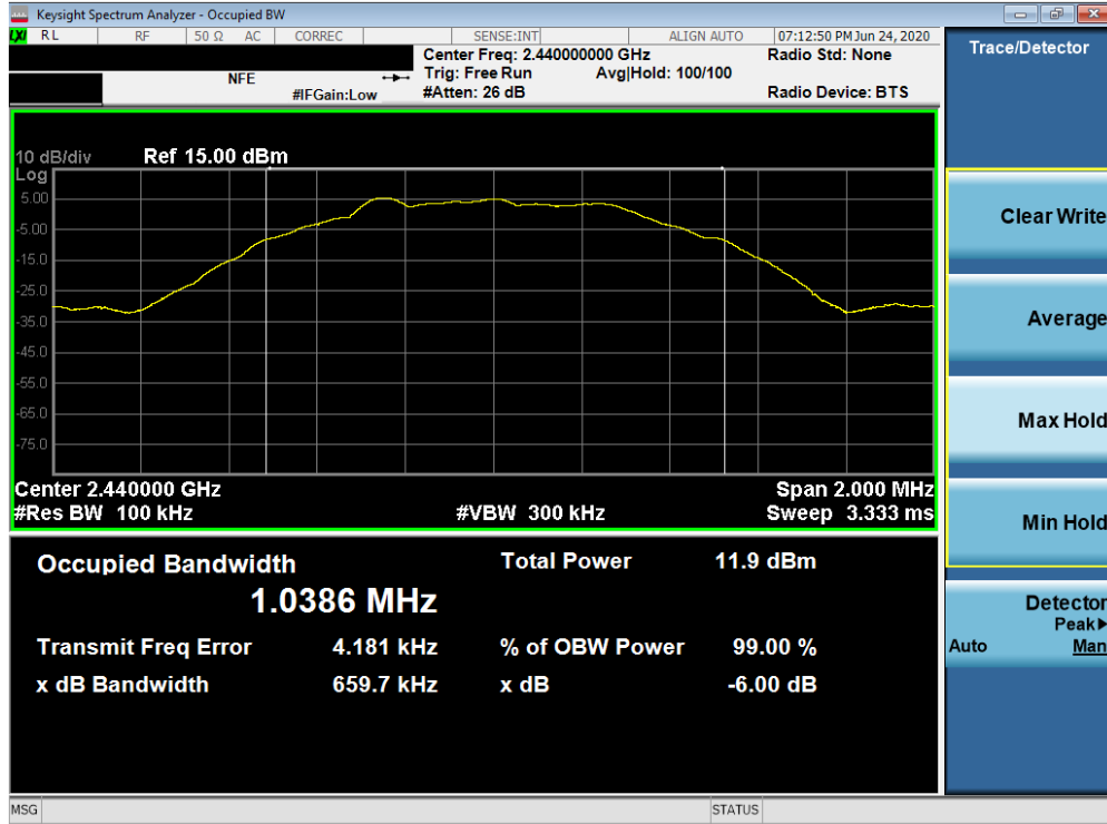
Plot 7-5. 6dB Bandwidth Plot (Bluetooth (LE), 500kbps – Ch. 19)
