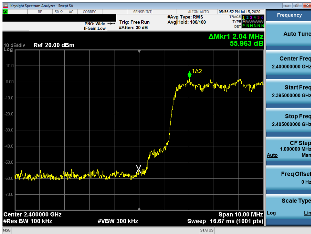
Plot 7-61. Band Edge Plot (Bluetooth with Hopping Enabled, 3 Mbps)
