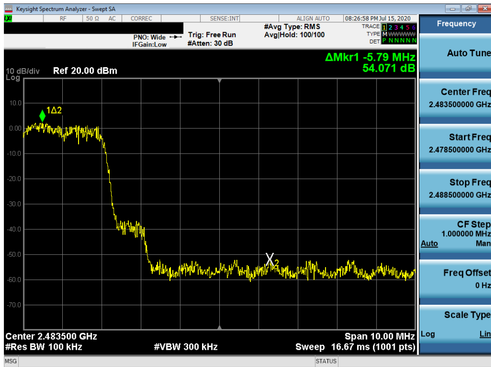
Plot 7-58. Band Edge Plot (Bluetooth with Hopping Enabled, 3 Mbps)
