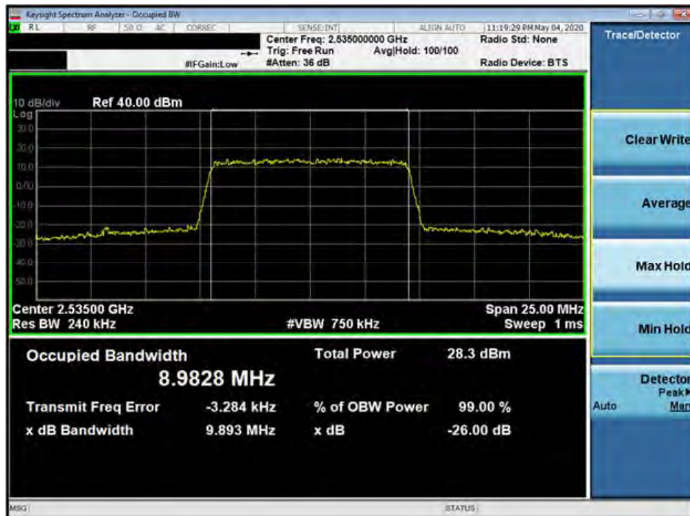
Plot 7-196. Occupied Bandwidth Plot (Band 7 - 10.0MHz 256-QAM - Full RB Configuration)
