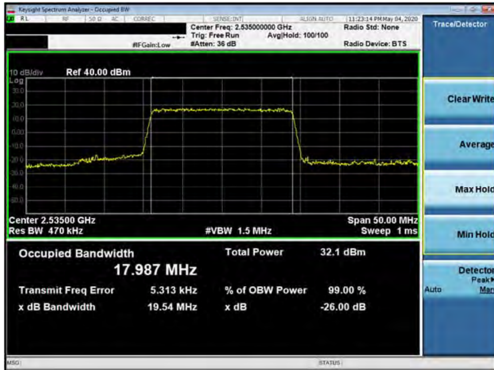
Plot 7-201. Occupied Bandwidth Plot (Band 7 - 20.0MHz QPSK - Full RB Configuration)
