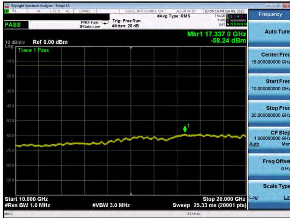
Plot 7-321. Conducted Spurious Plot (n66 - 20MHz DFT-s-OFDM-QPSK - RB Size 1, RB Offset 1 - High Channel)
