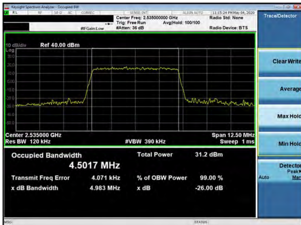
Plot 7-190. Occupied Bandwidth Plot (Band 7 - 5.0MHz 16-QAM - Full RB Configuration)
