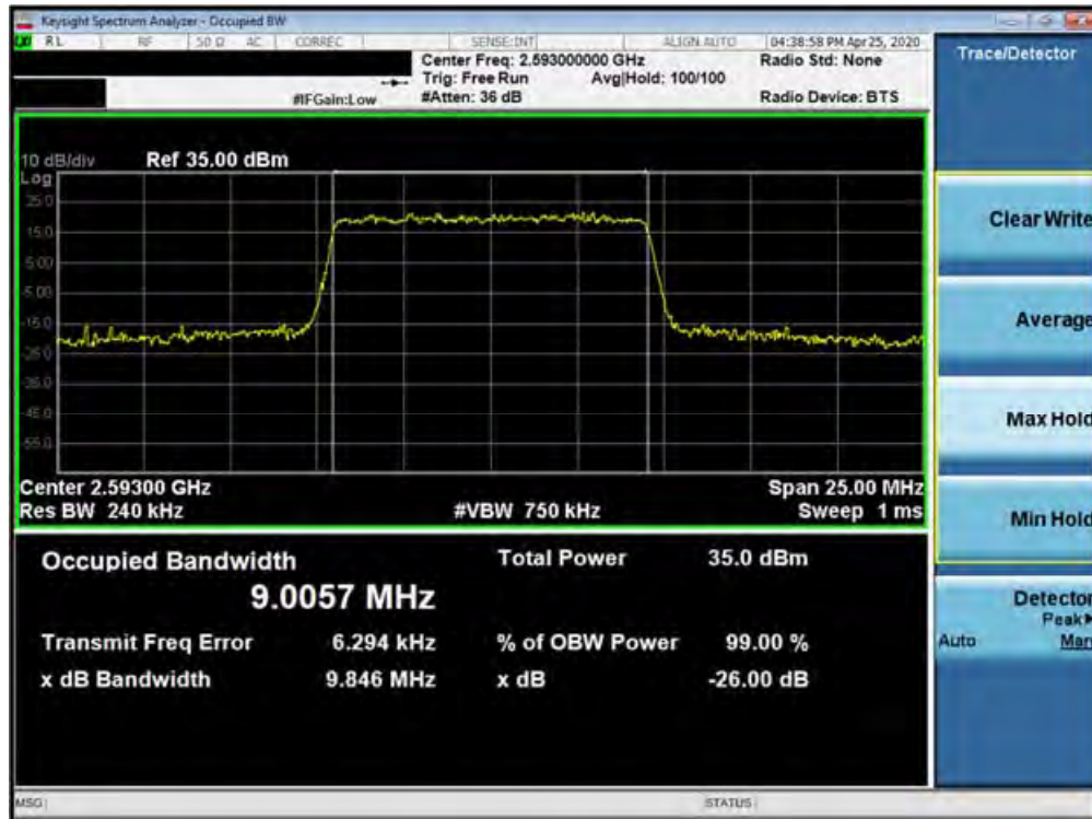
Plot 7-209. Occupied Bandwidth Plot (Band 41 (PC2) - 10.0MHz QPSK - Full RB Configuration)
