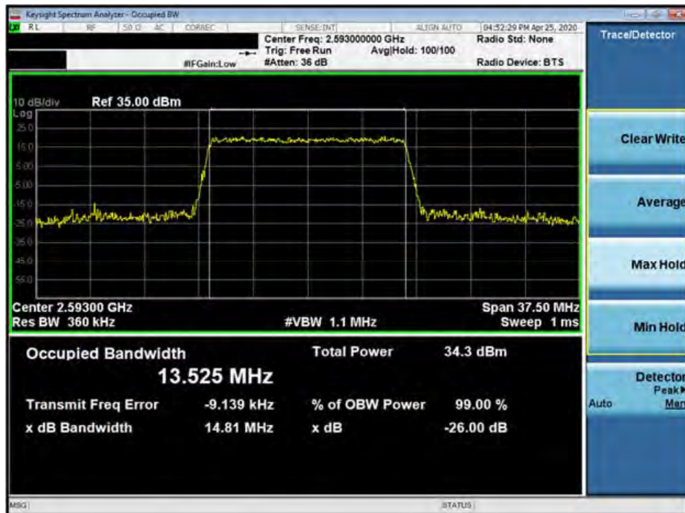
Plot 7-214. Occupied Bandwidth Plot (Band 41 (PC2) - 15.0MHz 16-QAM - Full RB Configuration)
