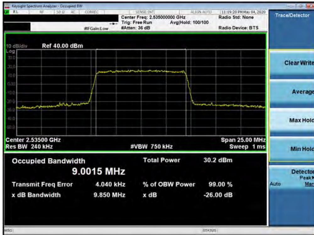
Plot 7-195. Occupied Bandwidth Plot (Band 7 - 10.0MHz 64-QAM - Full RB Configuration)
