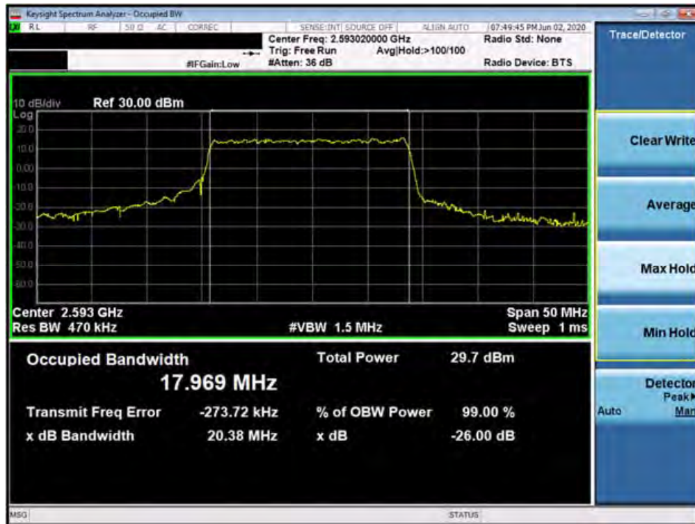
Plot 7-222. Occupied Bandwidth Plot (n41 20MHz QPSK-CP-OFDM - Full RB Configuration)
