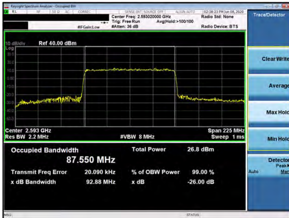
Plot 7-250. Occupied Bandwidth Plot (n41 90MHz 256QAM-CP-OFDM- Full RB Configuration)
