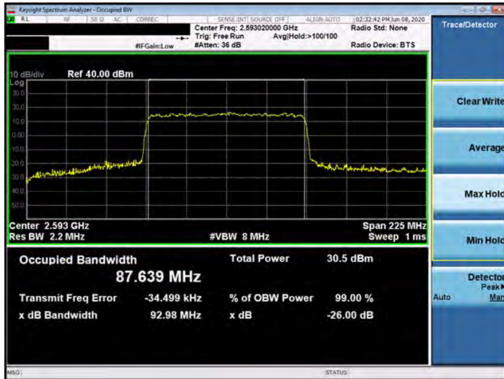
Plot 7-247. Occupied Bandwidth Plot (n41 90MHz QPSK-CP-OFDM - Full RB Configuration)
