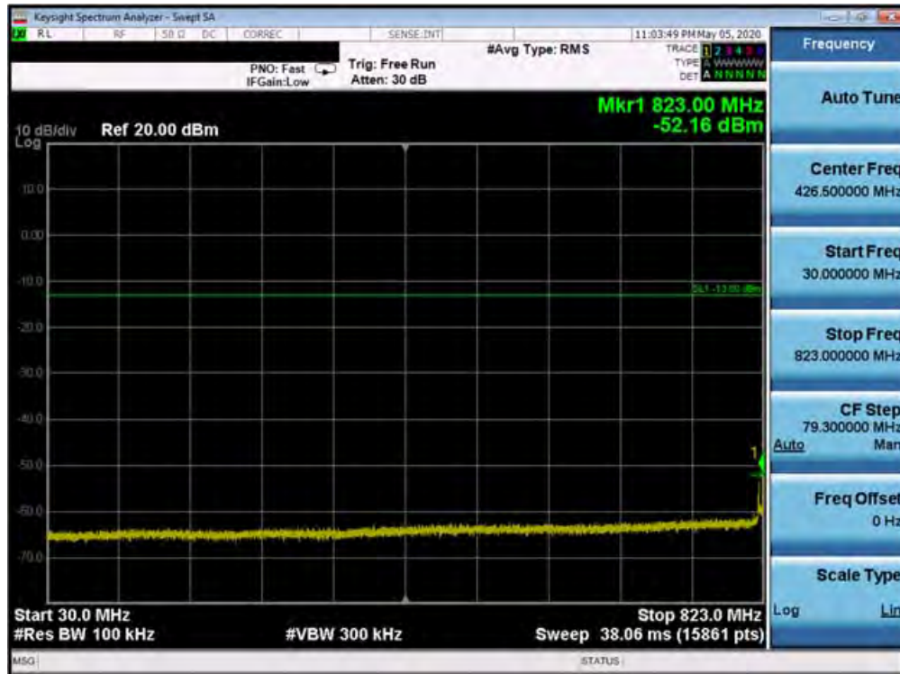
Plot 7-286. Conducted Spurious Plot (Band 26/5 - 10.0MHz QPSK - RB Size 1, RB Offset 0 - Low Channel)
