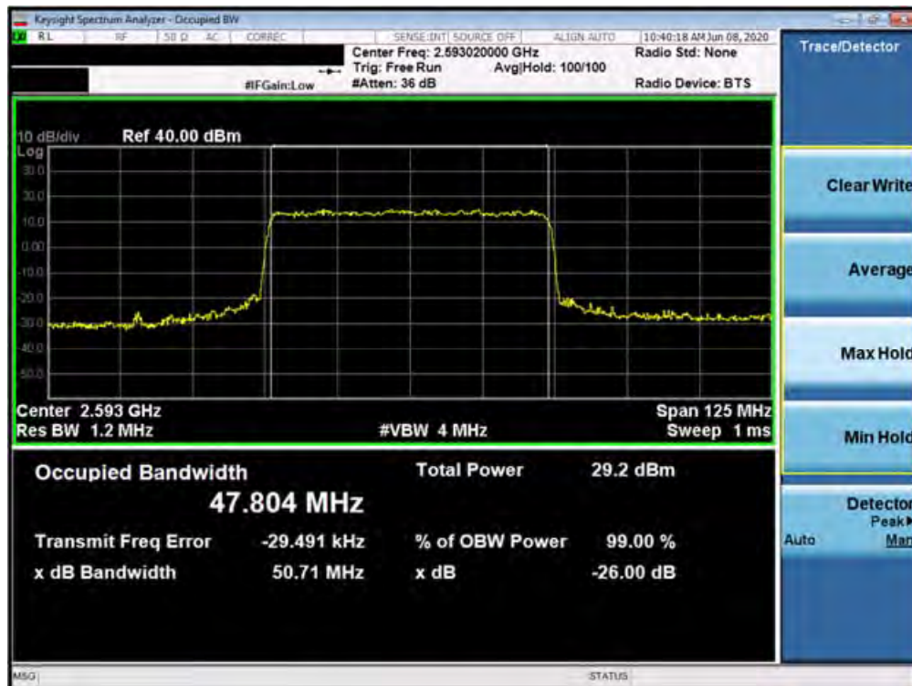
Plot 7-234. Occupied Bandwidth Plot (n41 50MHz 64QAM-CP-OFDM- Full RB Configuration)
