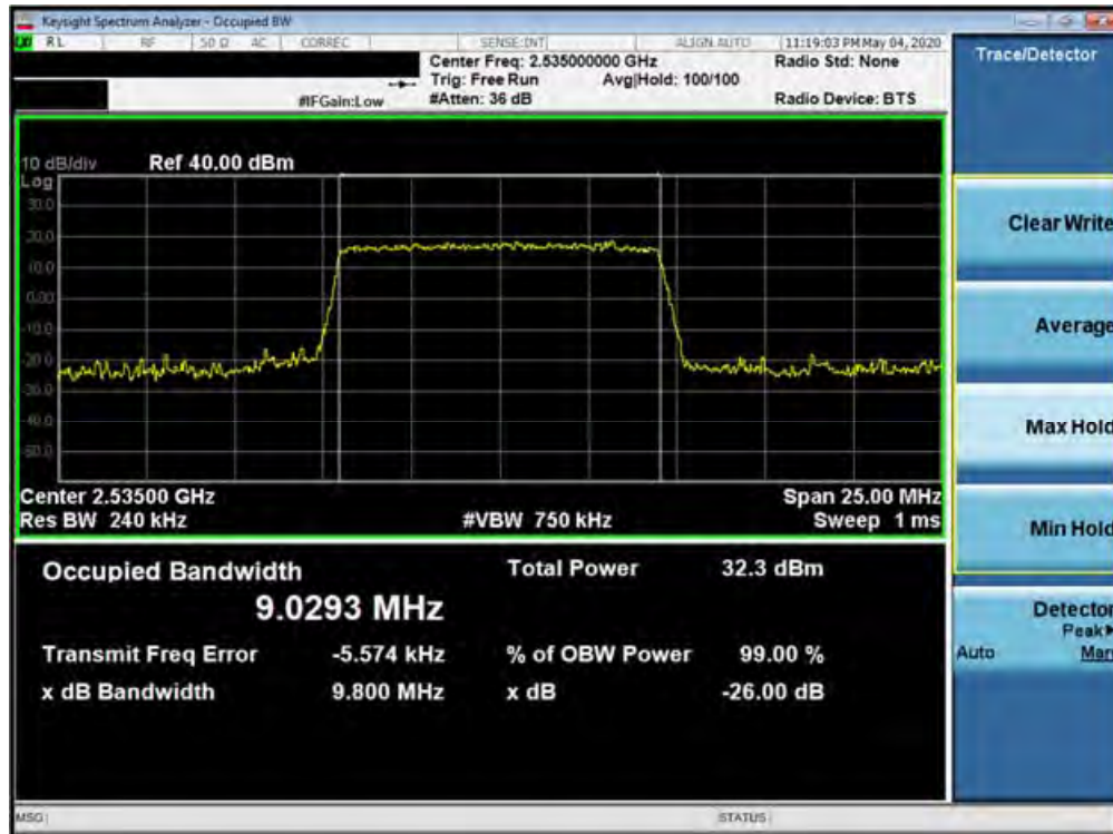
Plot 7-193. Occupied Bandwidth Plot (Band 7 - 10.0MHz QPSK - Full RB Configuration)
