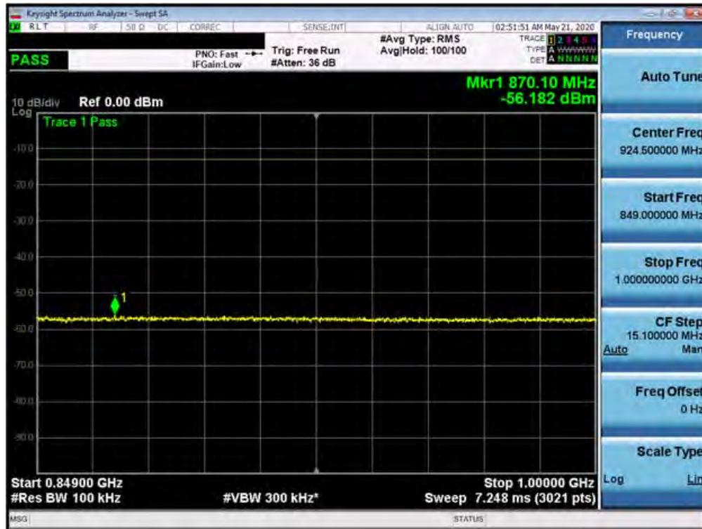
Plot 7-299. Conducted Spurious Plot (n5 - 20.0MHz DFT-s-OFDM BPSK - RB Size 1, RB Offset 0 - Mid Channel)
