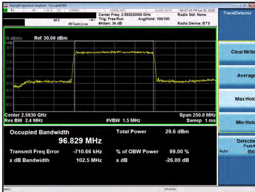
Plot 7-254. Occupied Bandwidth Plot (n41 100MHz 64QAM-CP-OFDM- Full RB Configuration)
