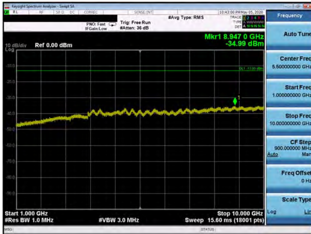
Plot 7-285. Conducted Spurious Plot (Band 13 - 10.0MHz QPSK - RB Size 1, RB Offset 0)
