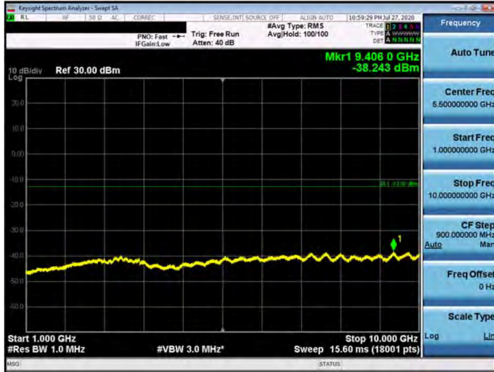
Plot 7-273. Conducted Spurious Plot (n71 - 20MHz DFT-s-OFDM-QPSK - RB Size 1, RB Offset 1 - High Channel)
