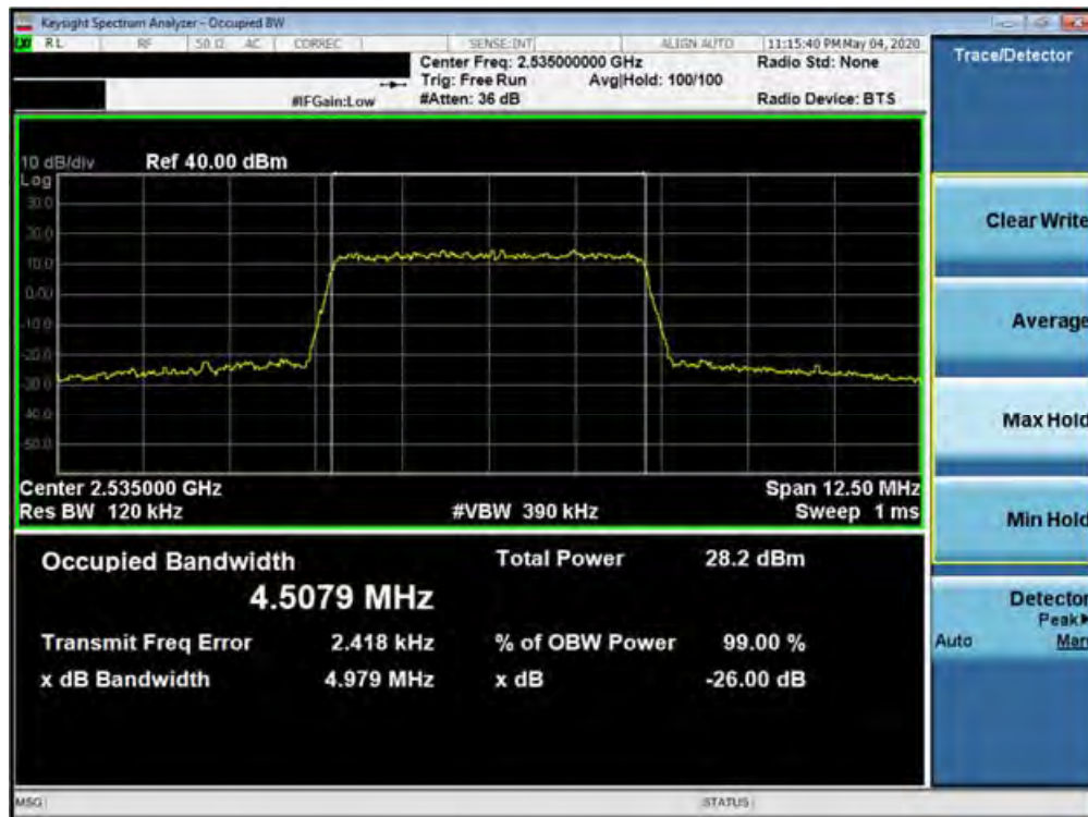
Plot 7-192. Occupied Bandwidth Plot (Band 7 - 5.0MHz 256-QAM - Full RB Configuration)
