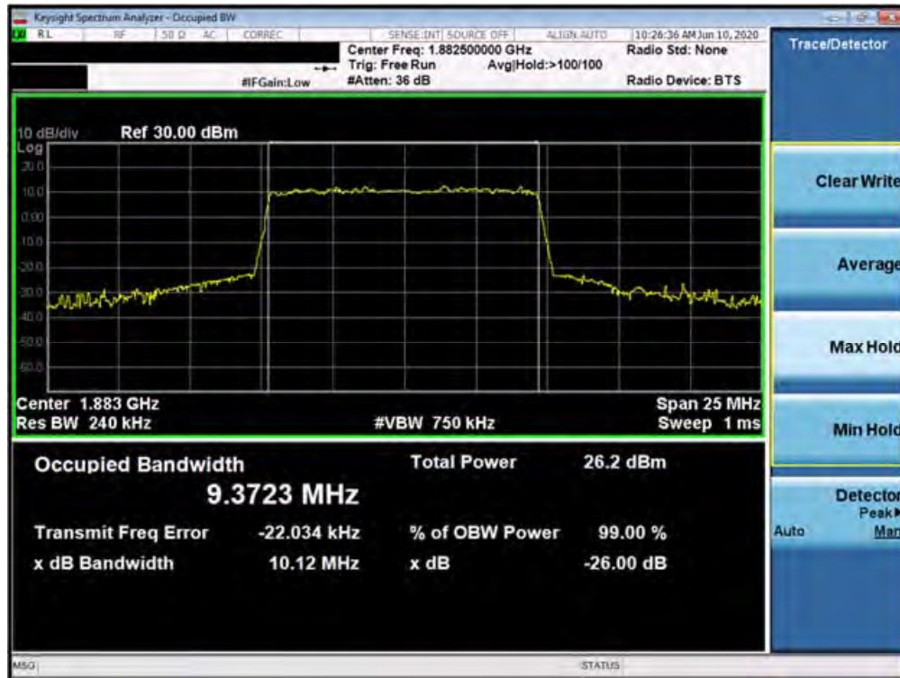
Plot 7-178. Occupied Bandwidth Plot (n25/2 10MHz 256QAM-CP-OFDM- Full RB Configuration)
