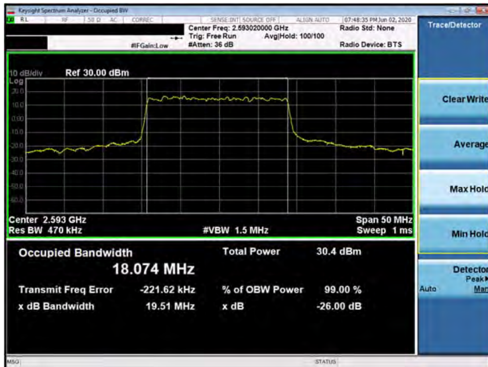
Plot 7-224. Occupied Bandwidth Plot (n41 20MHz 64QAM-CP-OFDM- Full RB Configuration)
