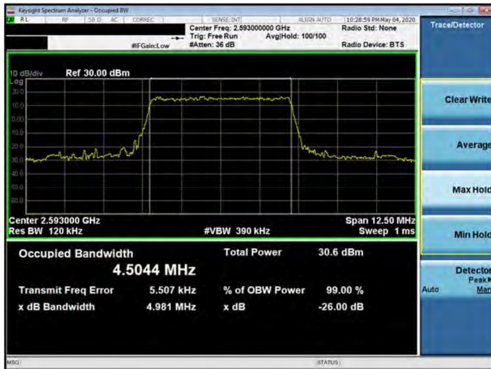
Plot 7-208. Occupied Bandwidth Plot (Band 41 (PC2) - 5.0MHz 256-QAM - Full RB Configuration)
