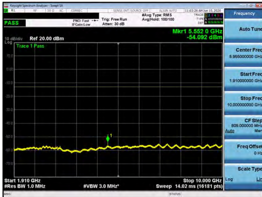
Plot 7-332. Conducted Spurious Plot (n25/2 - 20MHz DFT-s-OFDM-QPSK - RB Size 1, RB Offset 1 - Low Channel)
