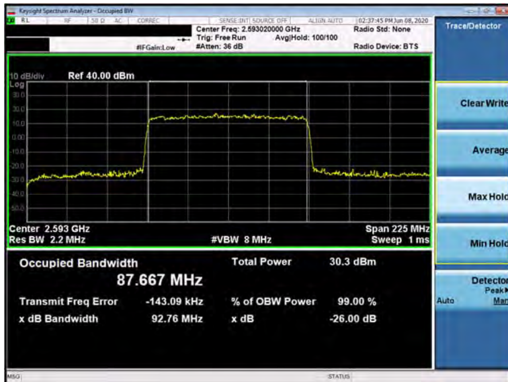
Plot 7-248. Occupied Bandwidth Plot (n41 90MHz 16QAM-CP-OFDM - Full RB Configuration)
