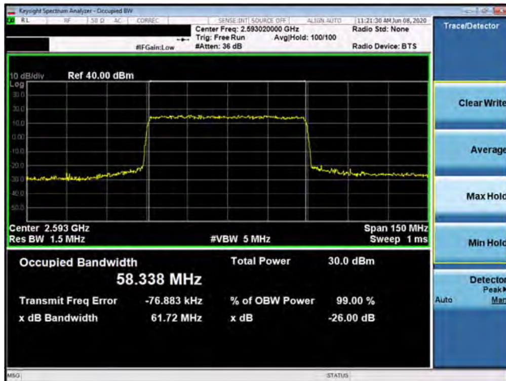
Plot 7-238. Occupied Bandwidth Plot (n41 60MHz 16QAM-CP-OFDM - Full RB Configuration)
