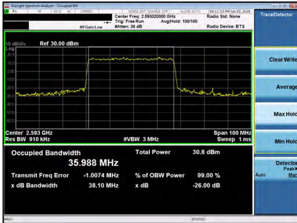
Plot 7-229. Occupied Bandwidth Plot (n41 40MHz 64QAM-CP-OFDM- Full RB Configuration)
