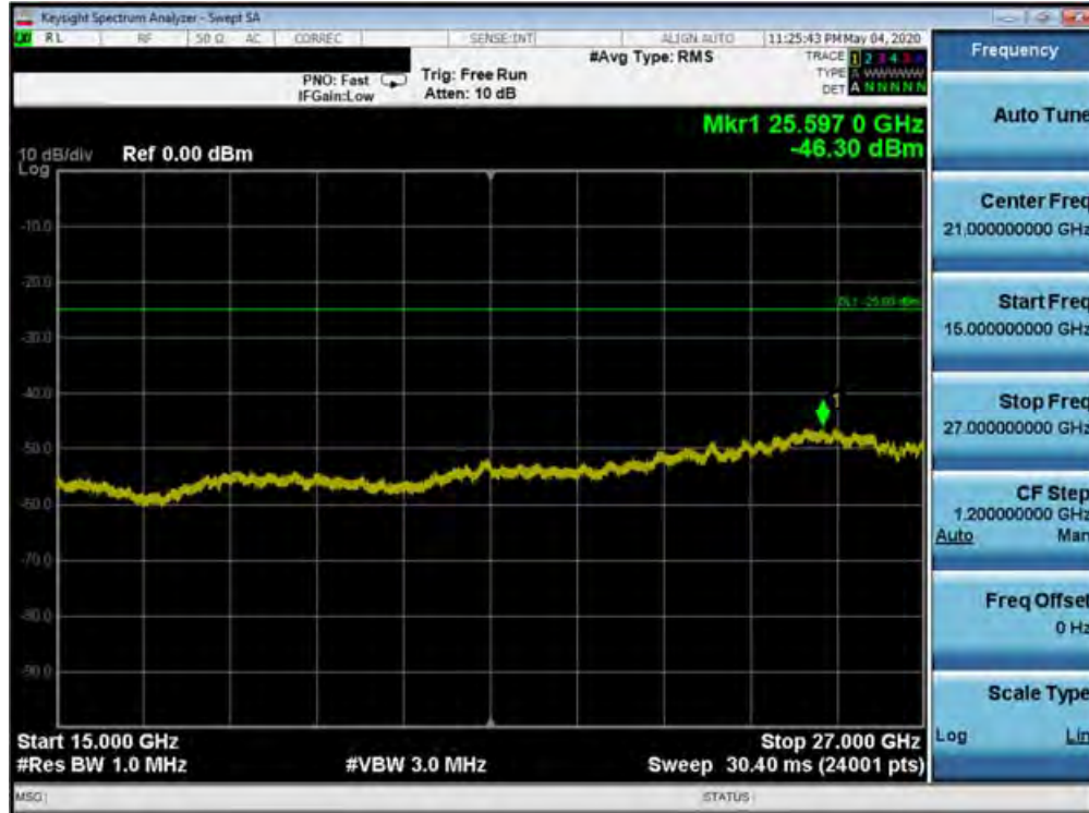
Plot 7-348. Conducted Spurious Plot (Band 7 - 20.0MHz QPSK - RB Size 1, RB Offset 0 - High Channel)
