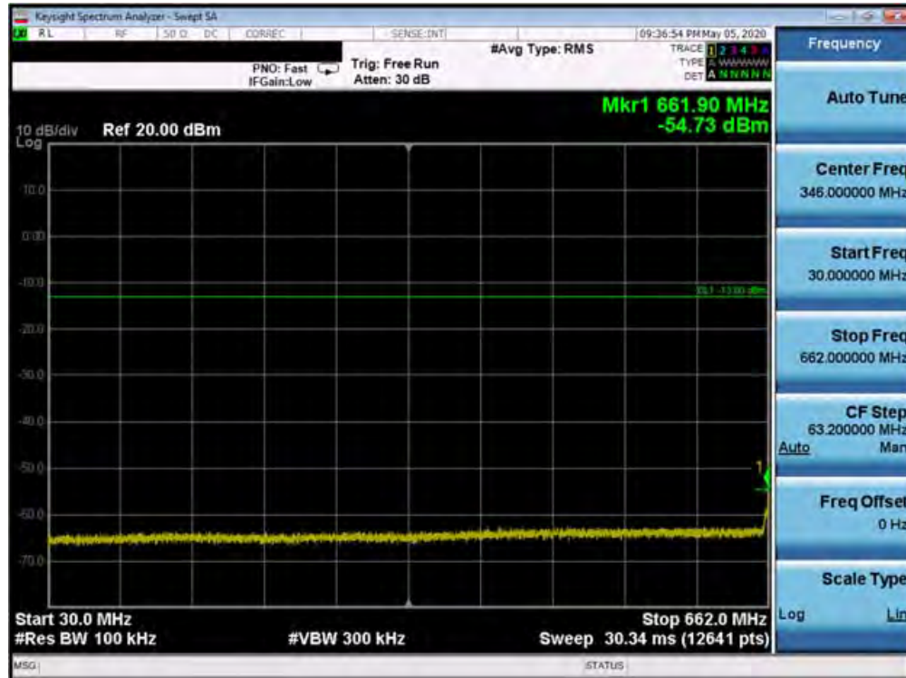
Plot 7-256. Conducted Spurious Plot (Band 71 - 20.0MHz QPSK - RB Size 1, RB Offset 0 - Low Channel)
