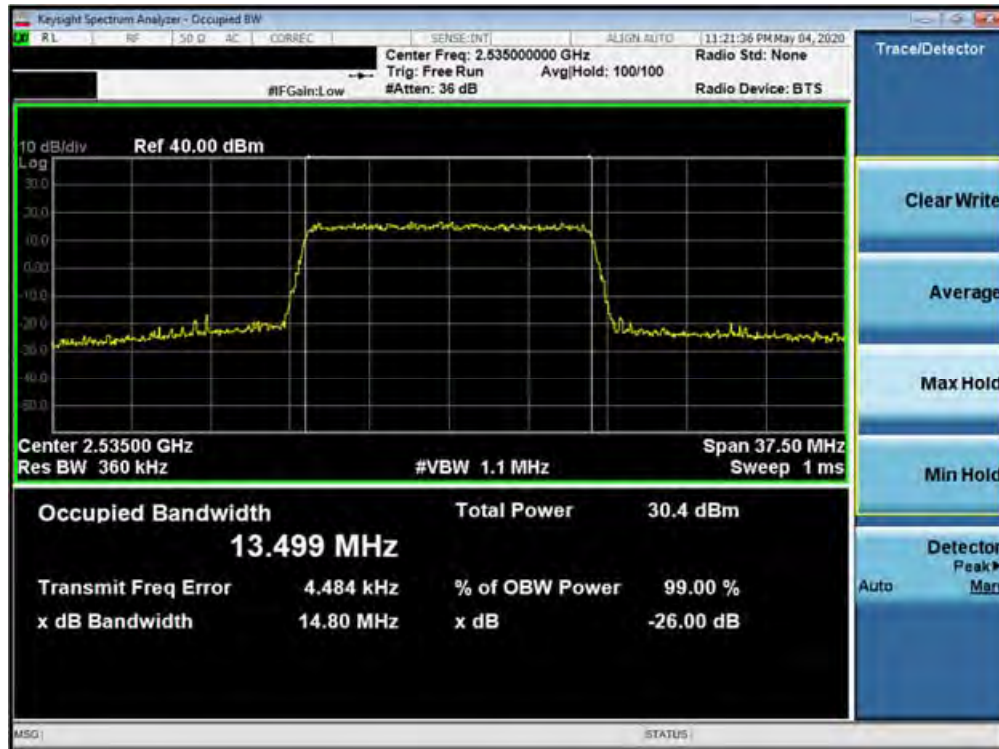
Plot 7-199. Occupied Bandwidth Plot (Band 7 - 15.0MHz 64-QAM - Full RB Configuration)
