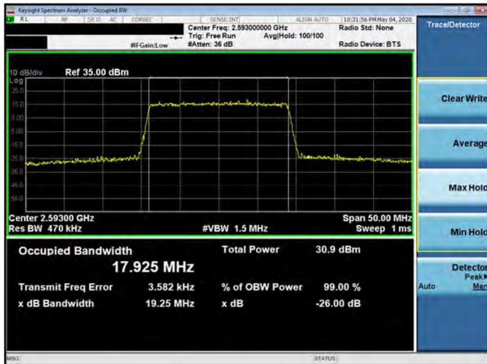
Plot 7-220. Occupied Bandwidth Plot (Band 41 (PC2) - 20.0MHz 256-QAM - Full RB Configuration)
