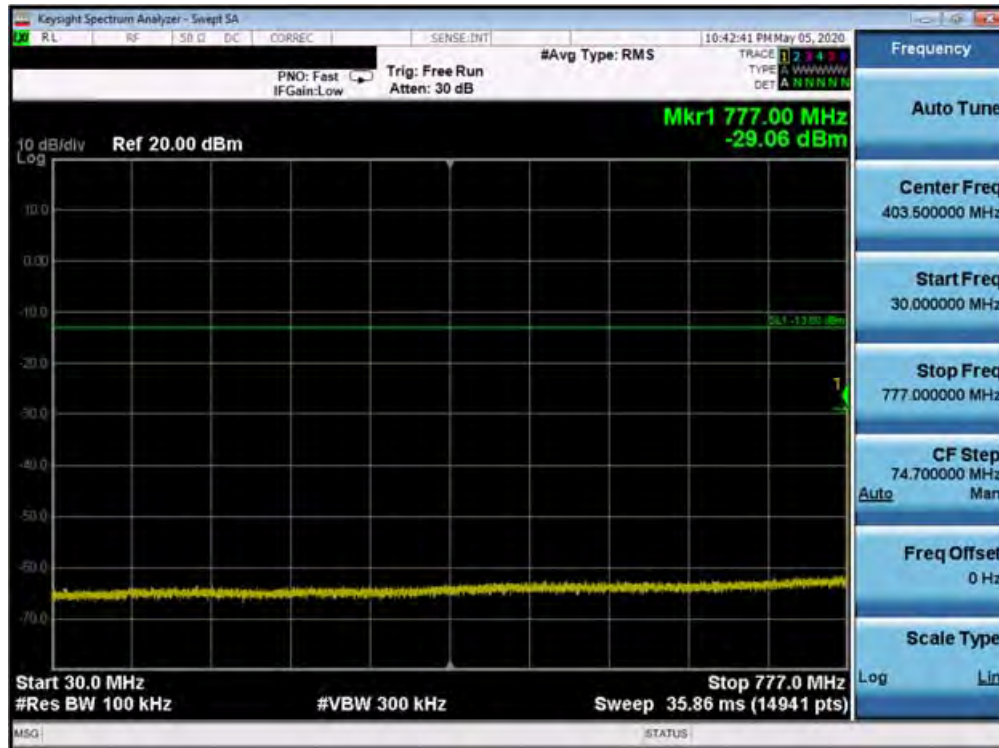
Plot 7-283. Conducted Spurious Plot (Band 13 - 10.0MHz QPSK - RB Size 1, RB Offset 0)
