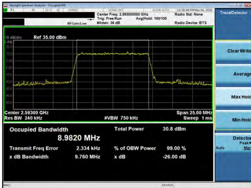
Plot 7-212. Occupied Bandwidth Plot (Band 41 (PC2) - 10.0MHz 256-QAM - Full RB Configuration)
