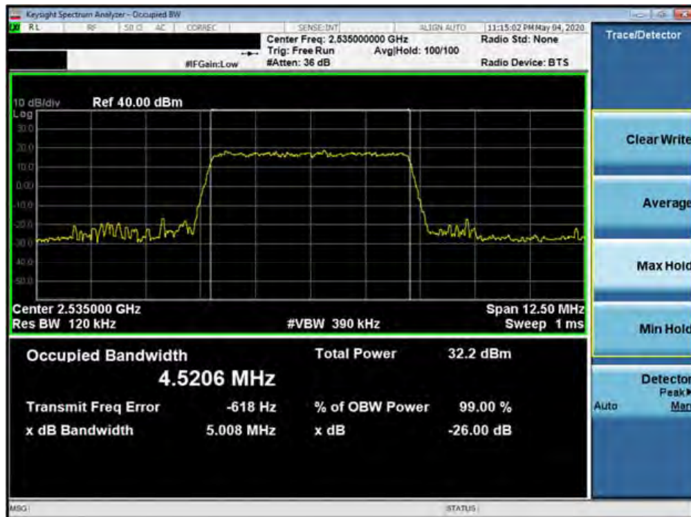
Plot 7-189. Occupied Bandwidth Plot (Band 7 - 5.0MHz QPSK - Full RB Configuration)
