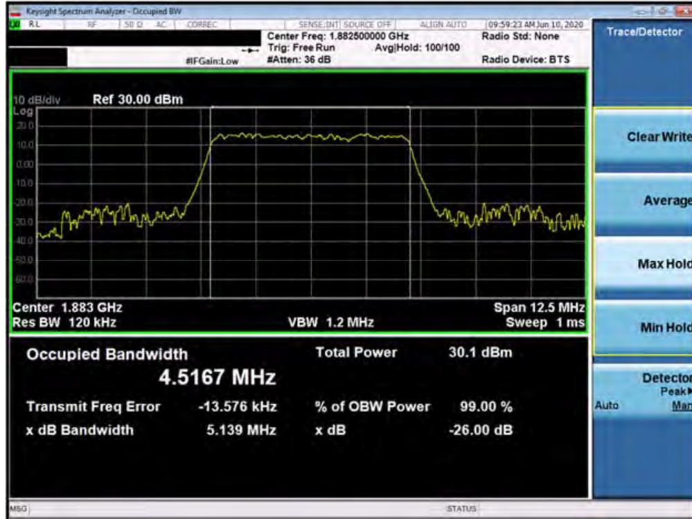
Plot 7-171. Occupied Bandwidth Plot (n25/2 5MHz 16QAM-CP-OFDM - Full RB Configuration)
