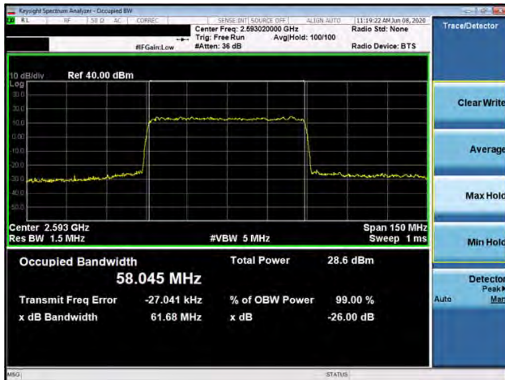
Plot 7-240. Occupied Bandwidth Plot (n41 60MHz 256QAM-CP-OFDM- Full RB Configuration)
