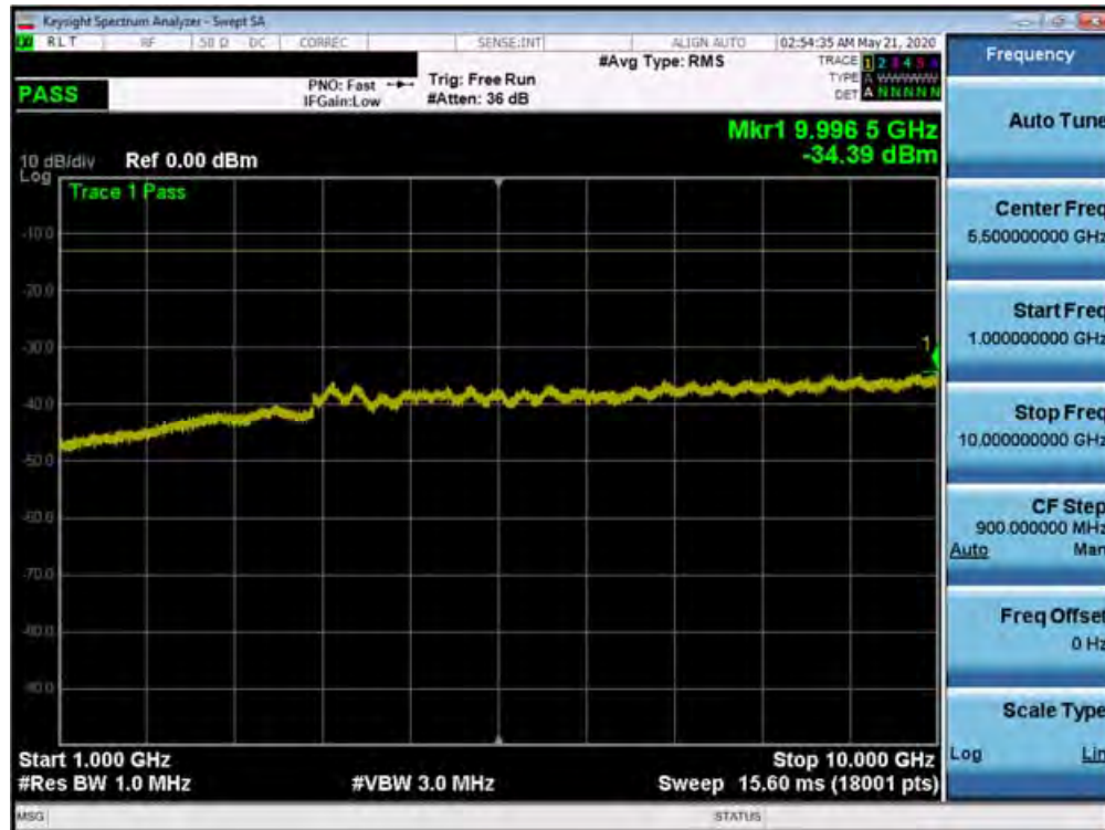
Plot 7-297. Conducted Spurious Plot (n5 - 20.0MHz DFT-s-OFDM BPSK - RB Size 1, RB Offset 0 - Low Channel)
