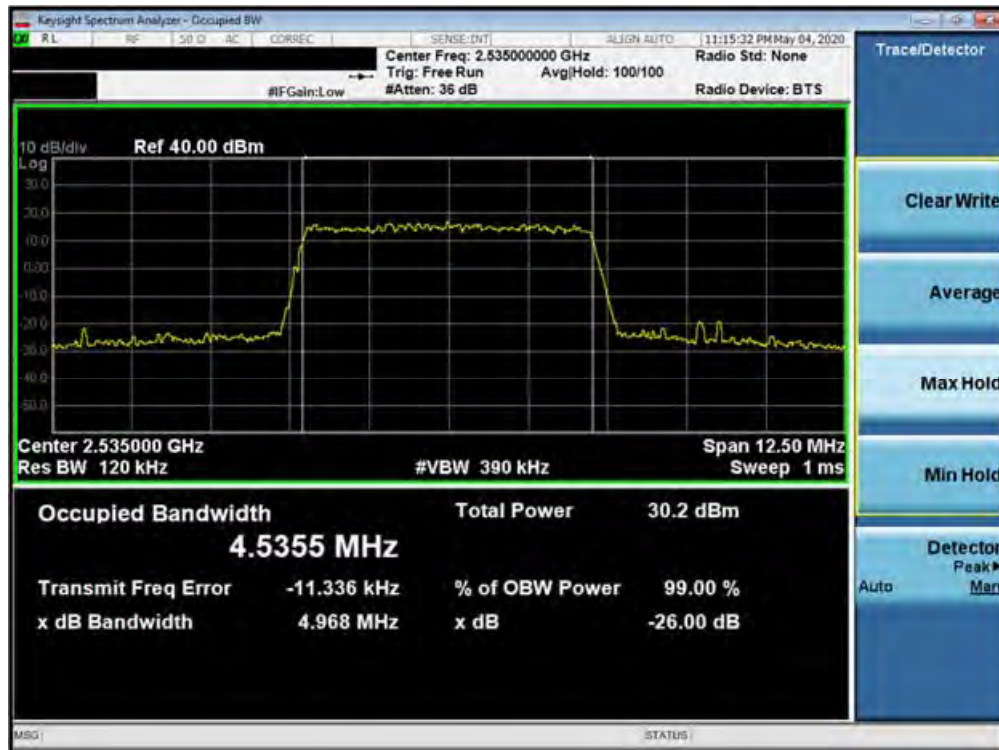
Plot 7-191. Occupied Bandwidth Plot (Band 7 - 5.0MHz 64-QAM - Full RB Configuration)
