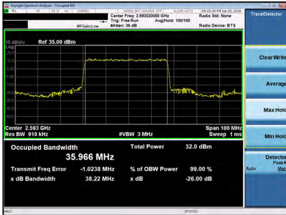
Plot 7-227. Occupied Bandwidth Plot (n41 40MHz QPSK-CP-OFDM - Full RB Configuration)
