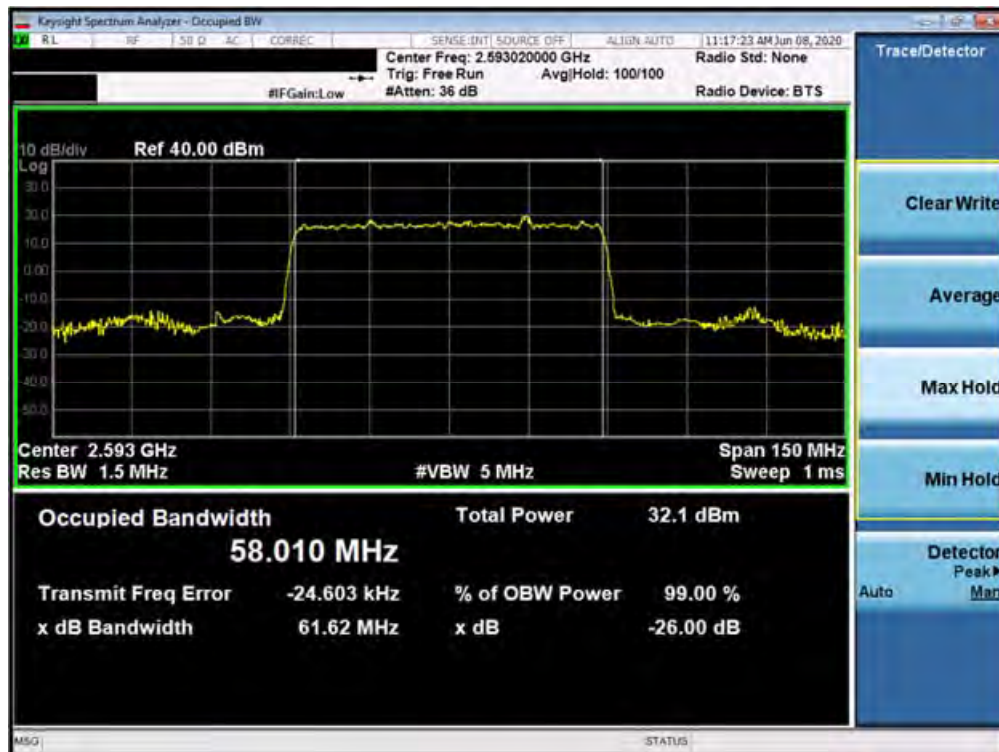
Plot 7-236. Occupied Bandwidth Plot (n41 60MHz BPSK-DFT-s-OFDM - Full RB Configuration)
