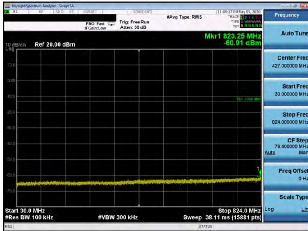
Plot 7-292. Conducted Spurious Plot (Band 26/5 - 10.0MHz QPSK - RB Size 1, RB Offset 0 - High Channel)
