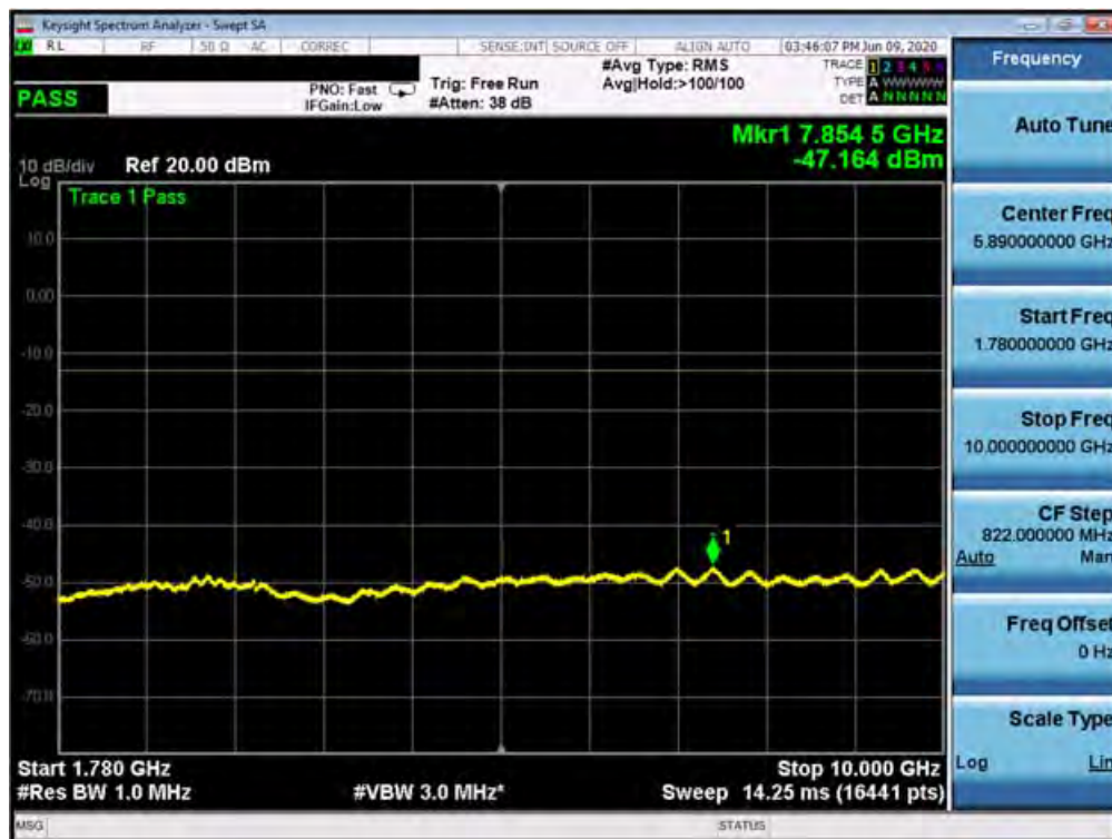
Plot 7-314. Conducted Spurious Plot (n66 - 20MHz DFT-s-OFDM-QPSK - RB Size 1, RB Offset 1 - Low Channel)
