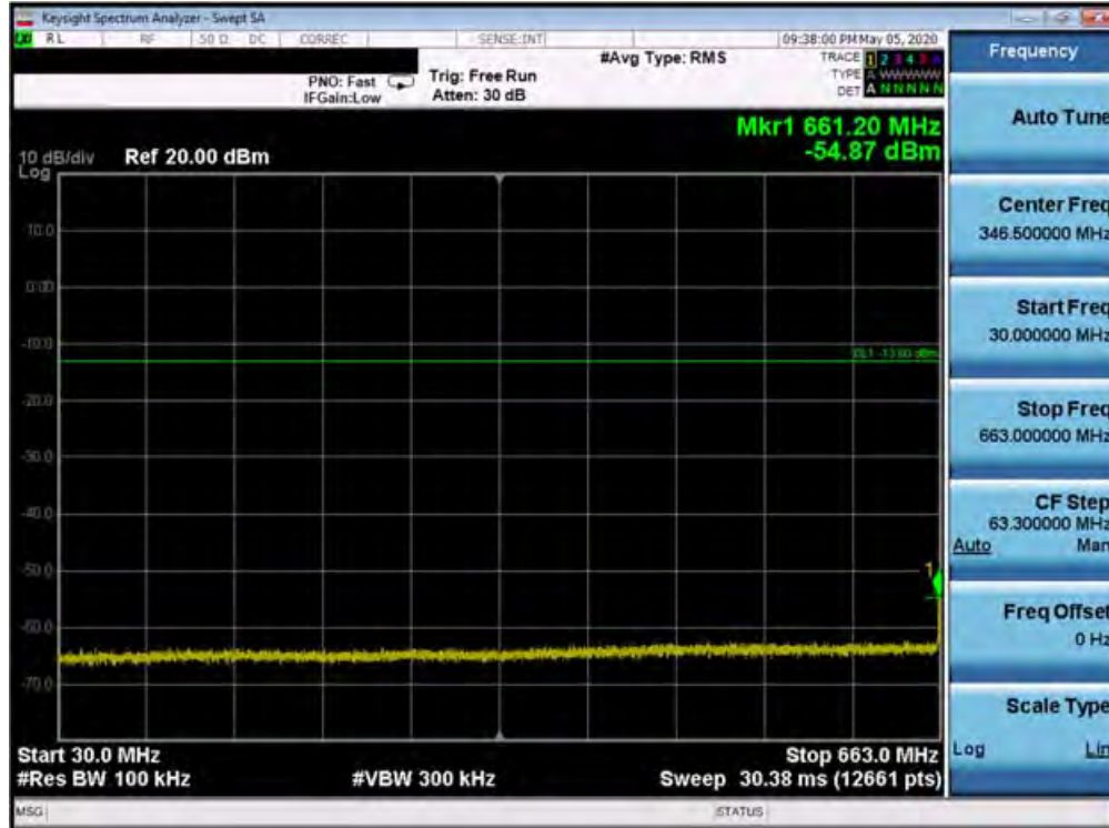
Plot 7-262. Conducted Spurious Plot (Band 71 - 20.0MHz QPSK - RB Size 1, RB Offset 0 - High Channel)
