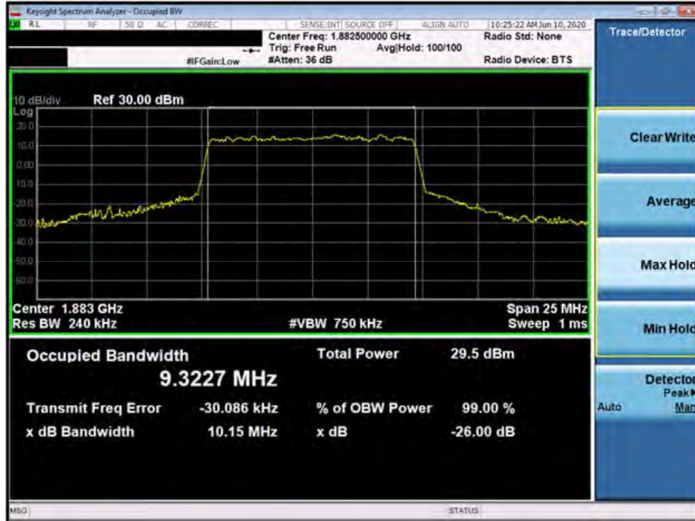
Plot 7-175. Occupied Bandwidth Plot (n25/2 10MHz QPSK-CP-OFDM - Full RB Configuration)
