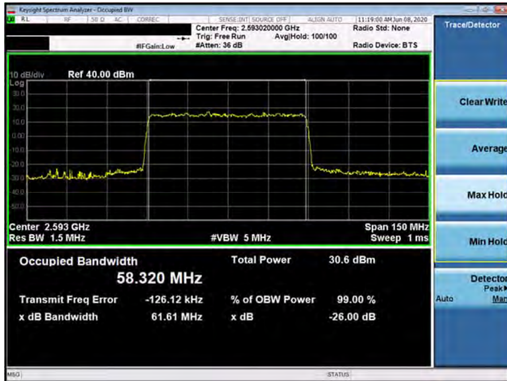
Plot 7-239. Occupied Bandwidth Plot (n41 60MHz 64QAM-CP-OFDM- Full RB Configuration)
