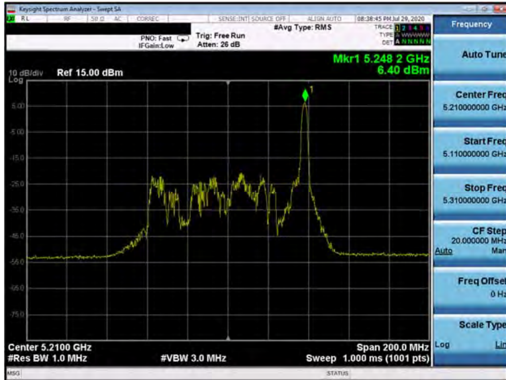
Plot 7-249. Power Spectral Density Plot MIMO ANT2 (80MHz BW 802.11ax – 26 Tones (UNII Band 1) – Ch. 42)
