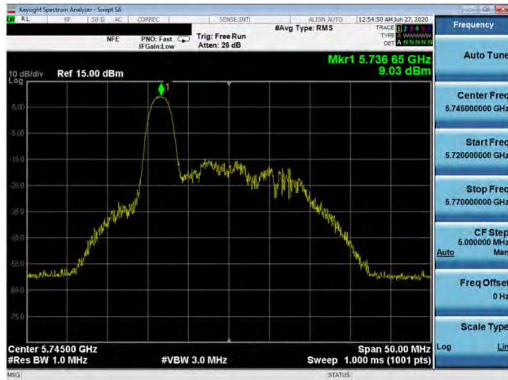
Plot 7-265. Power Spectral Density Plot MIMO ANT2 (20MHz BW 802.11ax – 26 Tones (UNII Band 3) – Ch. 149)
