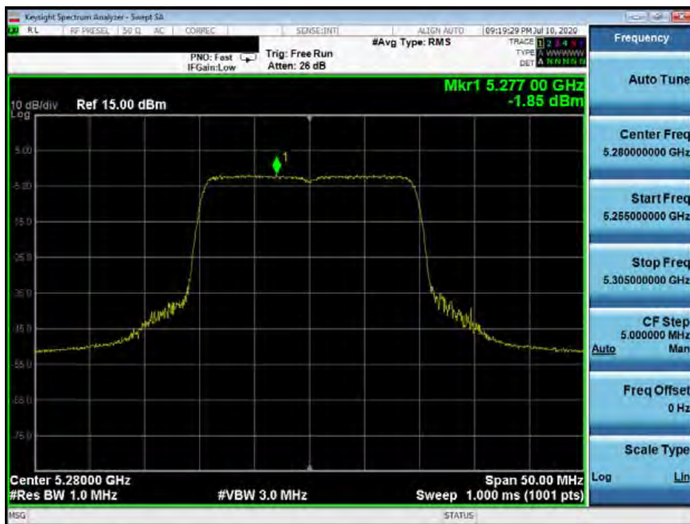
Plot 7-197. Power Spectral Density Plot SISO ANT2 (20MHz BW 802.11ax – Full Tones (UNII Band 2A) – Ch. 56)
