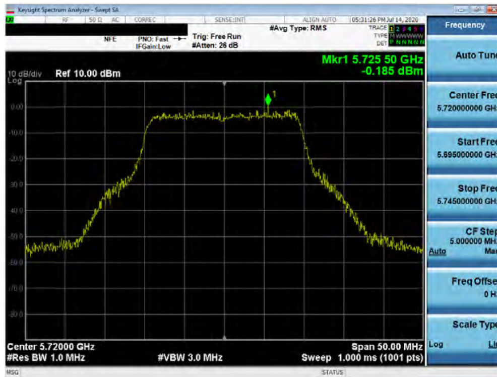
Plot 7-204. Power Spectral Density Plot SISO ANT2 (20MHz BW 802.11ax – Full Tones (UNII Band 2C) – Ch. 144)
