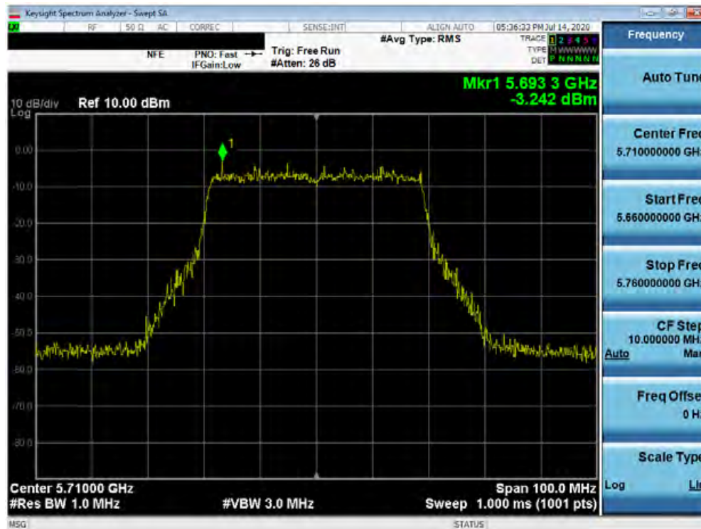
Plot 7-207. Power Spectral Density Plot SISO ANT2 (40MHz BW 802.11ax - Full Tones (UNII Band 2C) - Ch. 142)
