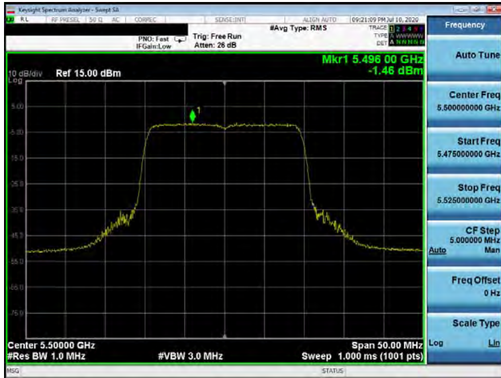
Plot 7-202. Power Spectral Density Plot SISO ANT2 (20MHz BW 802.11ax – Full Tones (UNII Band 2C) – Ch. 100)
