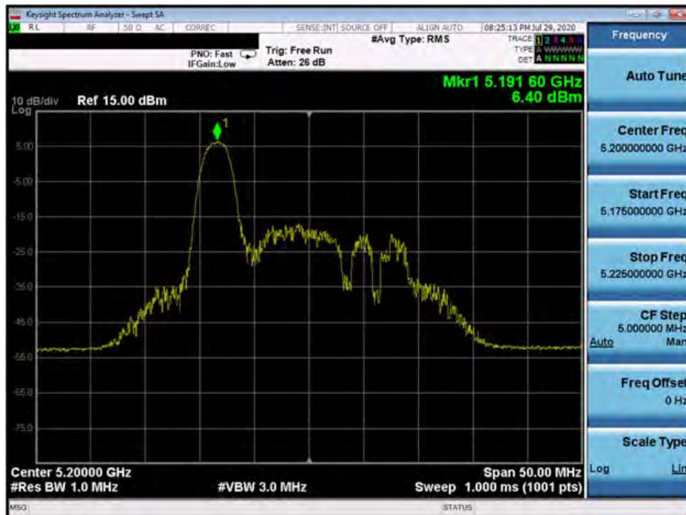
Plot 7-218. Power Spectral Density Plot MIMO ANT1 (20MHz BW 802.11ax – 26 Tones (UNII Band 1) – Ch. 40)
