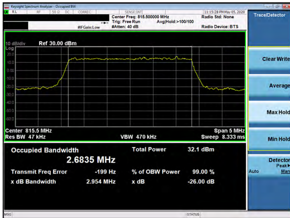
Plot 7-13. Occupied Bandwidth Plot (LTE Band 26 - 3MHz QPSK - Full RB Configuration)
