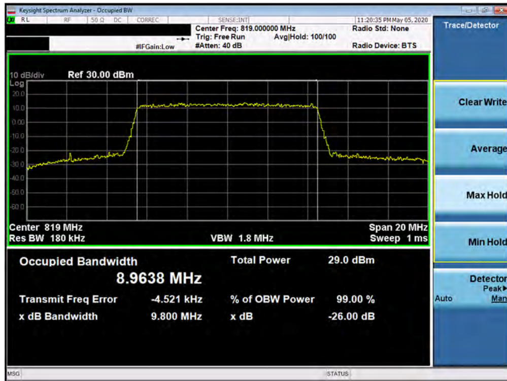
Plot 7-7. Occupied Bandwidth Plot (LTE Band 26 - 10MHz 64-QAM - Full RB Configuration)
