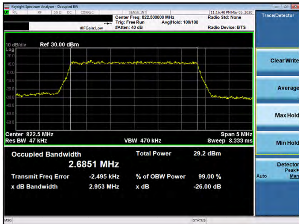
Plot 7-15. Occupied Bandwidth Plot (LTE Band 26 - 3MHz 64-QAM - Full RB Configuration)
