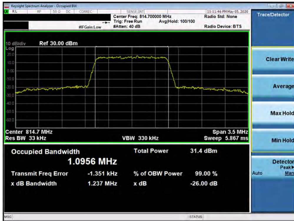
Plot 7-17. Occupied Bandwidth Plot (LTE Band 26 - 1.4MHz QPSK - Full RB Configuration)
