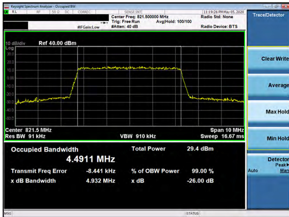
Plot 7-11. Occupied Bandwidth Plot (LTE Band 26 - 5MHz 64-QAM - Full RB Configuration)
