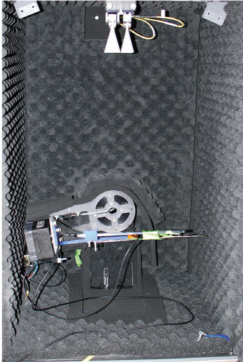
Test Setup Photo 7 – Radiated Power Measurement Setup (Figure 7-1)
