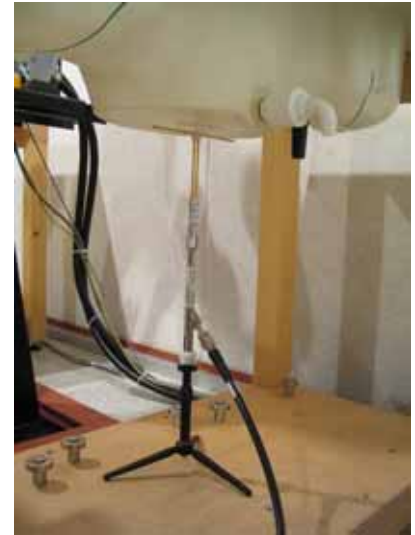
Photo of the dipole Antenna
