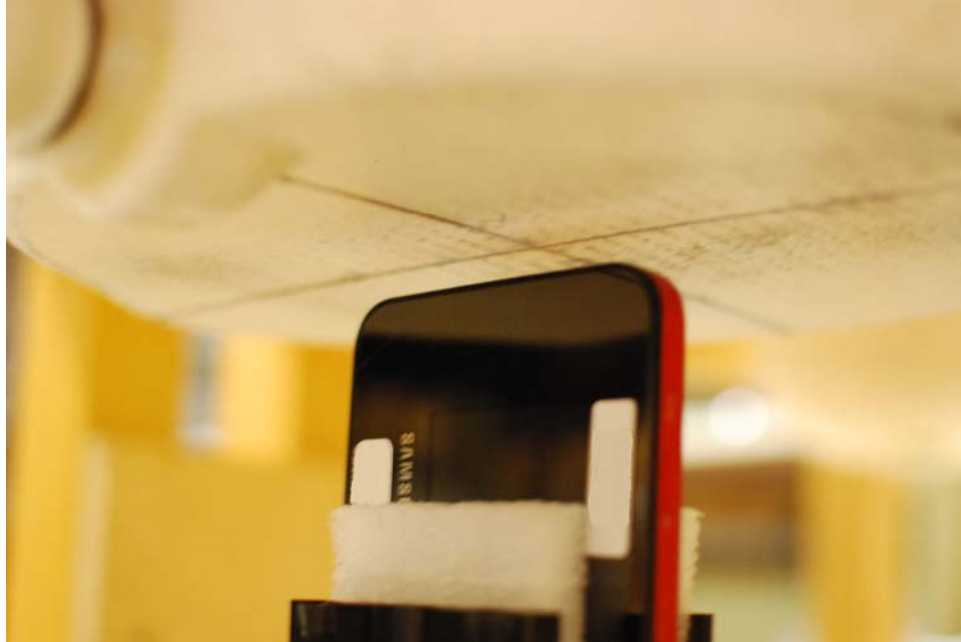
SAR Test Setup Photo 5 - Left Edge at 10 mm
