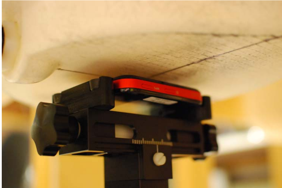
SAR Test Setup Photo 1 - Back Side at 10 mm
