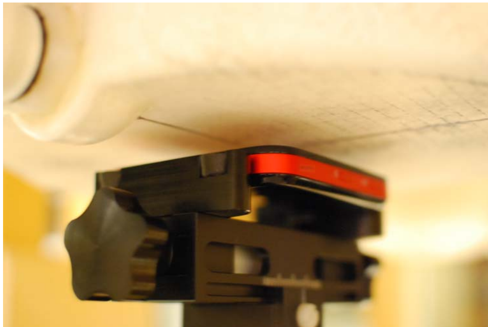
SAR Test Setup Photo 2 - Front Side at 10 mm
