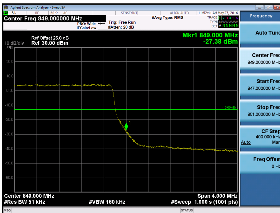
BAND 5. Upper Band Edge Plot (5M BW Ch.20625 QPSK RB25_Offset 0)
