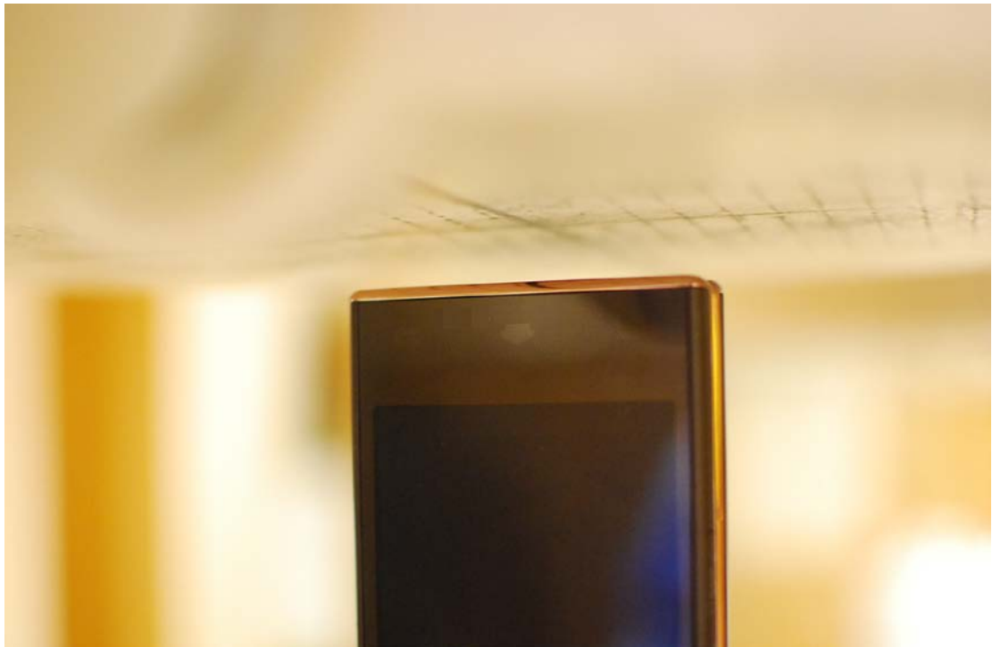
SAR Test Setup Photo 8 - Bottom Edge at 10 mm
