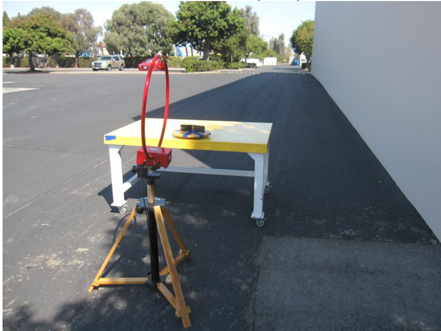
RADIATED EMISSIONS BELOW 30MHz (BACK)
