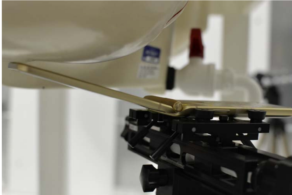
SAR Test Setup Photo 3 – Right Tilt
